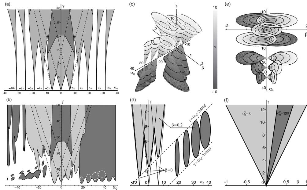
**Fig. 1**  $l = 0, \Delta\alpha(r) = \cos(4\pi r)$ : (a) Arnold's tongues corresponding to the decaying (light gray) and growing (dark gray) oscillations of the magnetic field with their linear approximation (dashed lines) for (a)  $\beta = 0$  and (b)  $\beta = 0.2$ ; 3D cones of the principal resonances with inclination determined by the Krein signature of the double eigenvalues (c) and their projections and cross-sections (d)-(f).
