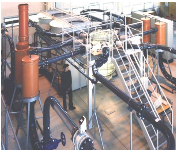
Fig. 1: View on the test facility ROCOM with the RPV model made from acryl
