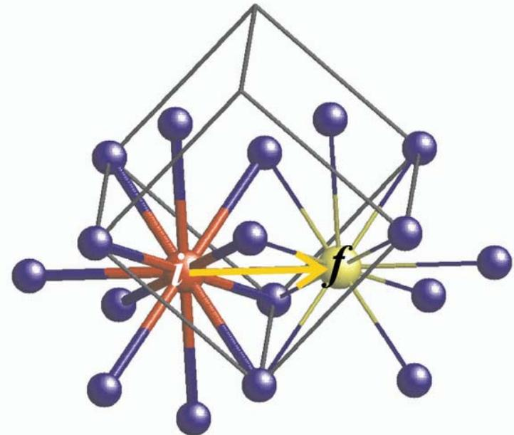
The jump configuration in an fcc lattice.
