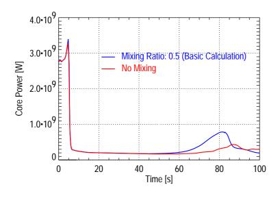
Fig. 5: Core Power in the different point kinetics calculations
