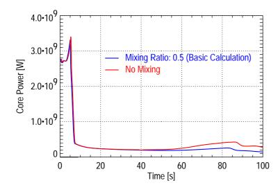
Fig. 2: Core power in the different DYN3D/ATHLET calculations
