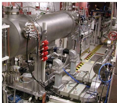
The warm window is made from polystyrene (Rexolite®) which is not very common as RF window material in accelerators. The window is a standard microwave part for WR650 waveguides. This gives a mechanically very simple and cost effective window design compared to ceramic windows.
