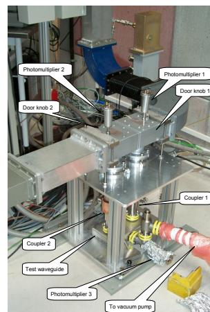
For coupler training a special test waveguide was used. The couplers were trained at room temperature with full reflection for all phases (4 steps with 30° step width). Only the antenna side was in vacuum.
