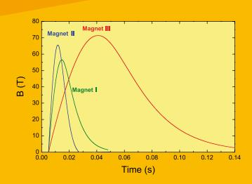
At the moment, the HLD operates three types of user magnets with the above shown temporal field profiles. In combination with these magnets, the experimental techniques listed below are available for users.
