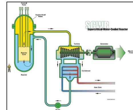
→ **fast neutron** induced fission is used to produce electrical power and to **burn up long lived actinides**
