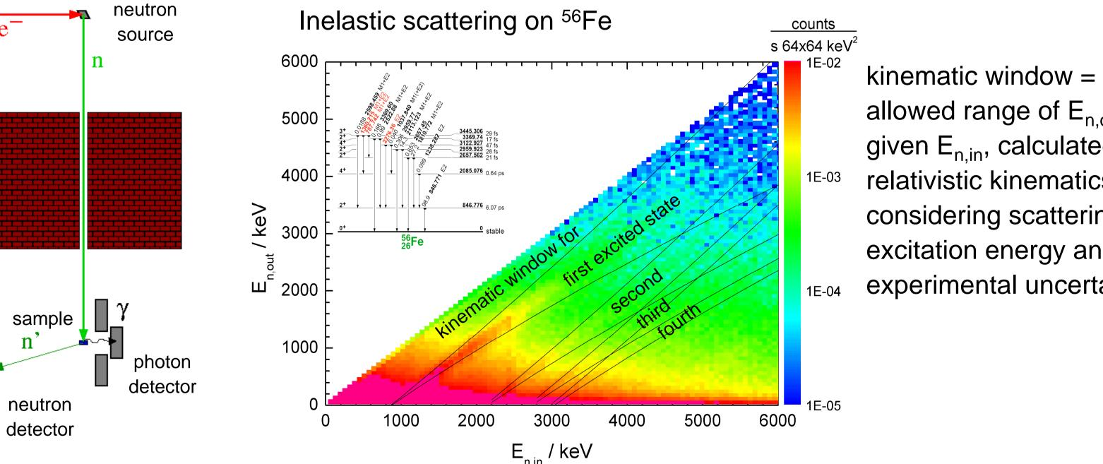
allowed range of  $E_{n,out}$  for given  $E_{n,in}$ , calculated in relativistic kinematics considering scattering angle, excitation energy and experimental uncertainties
