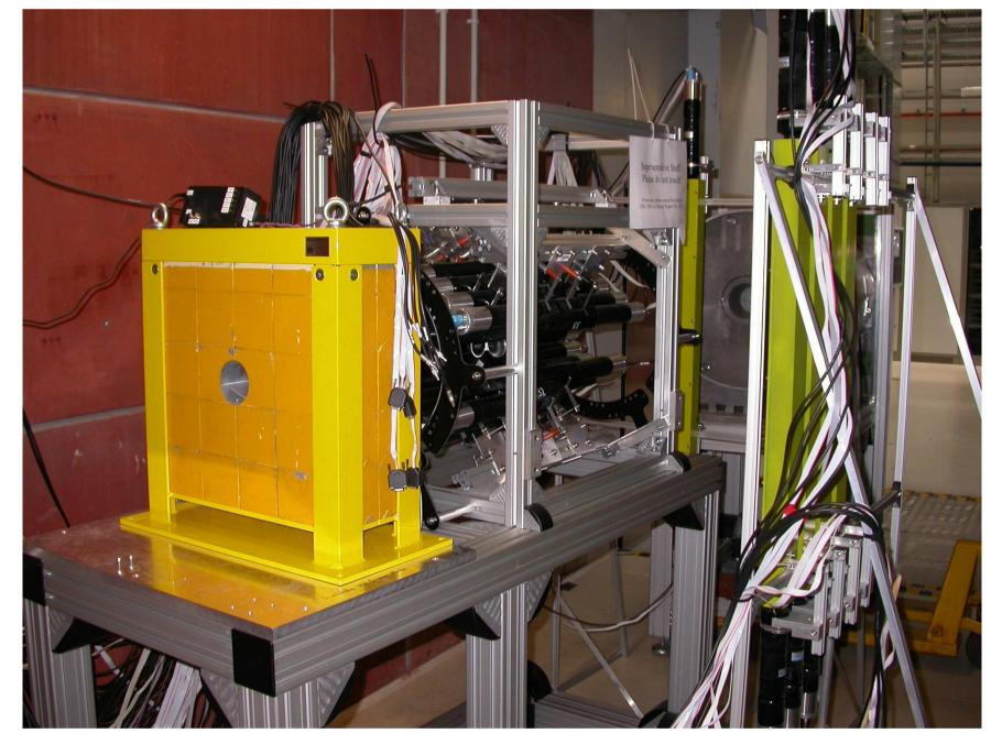
The nELBE detector setup: - 5 plastic scintillation detectors to detect the neutrons - an array of up to 42 BaF<sub>2</sub> crystals for photon detection
