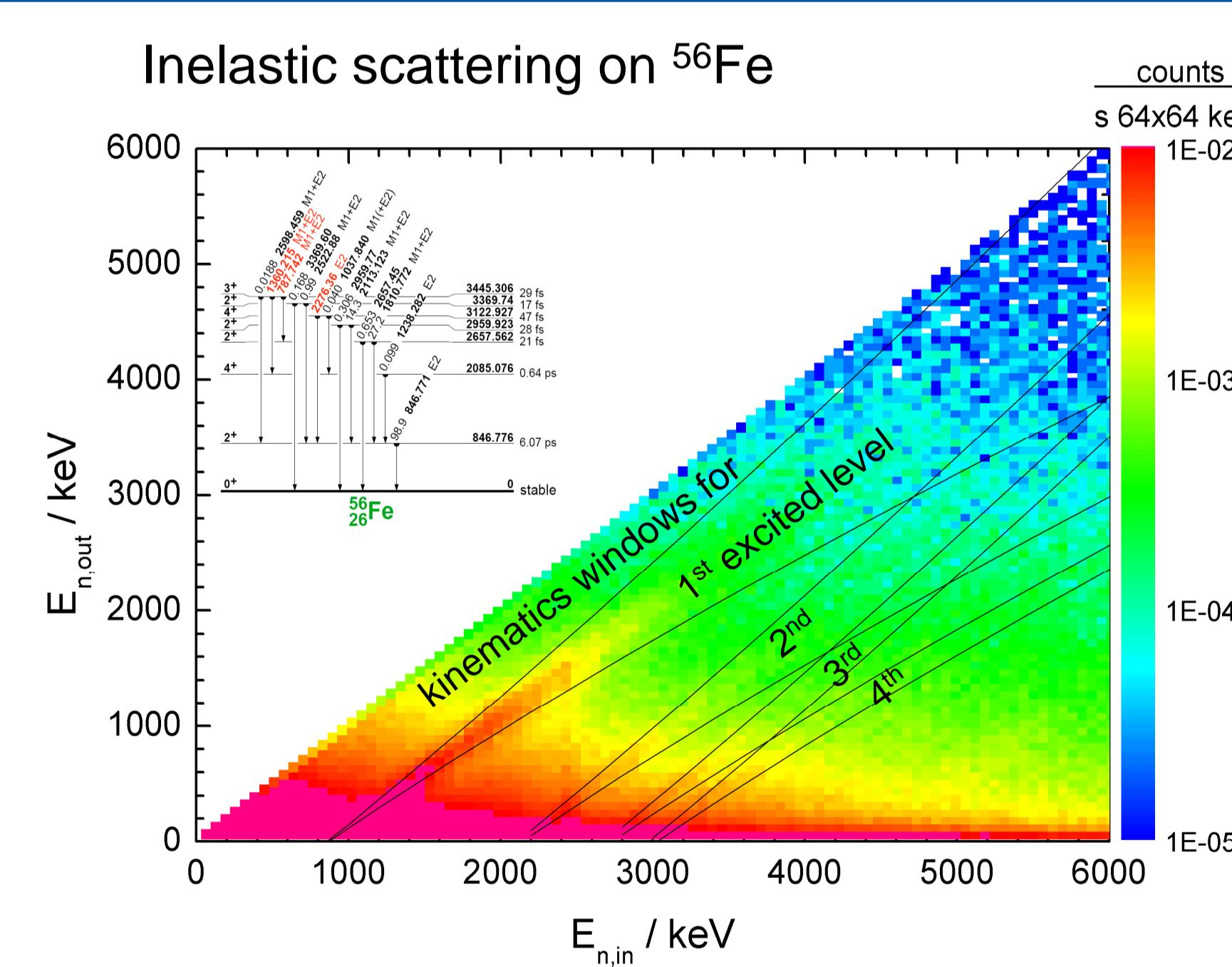
kinematics windows = possible range of E<sub>n,out</sub> for given E<sub>n,in</sub>, calculated by relativistic kinematics including scattering angle, excitation energy and experimental uncertainties
