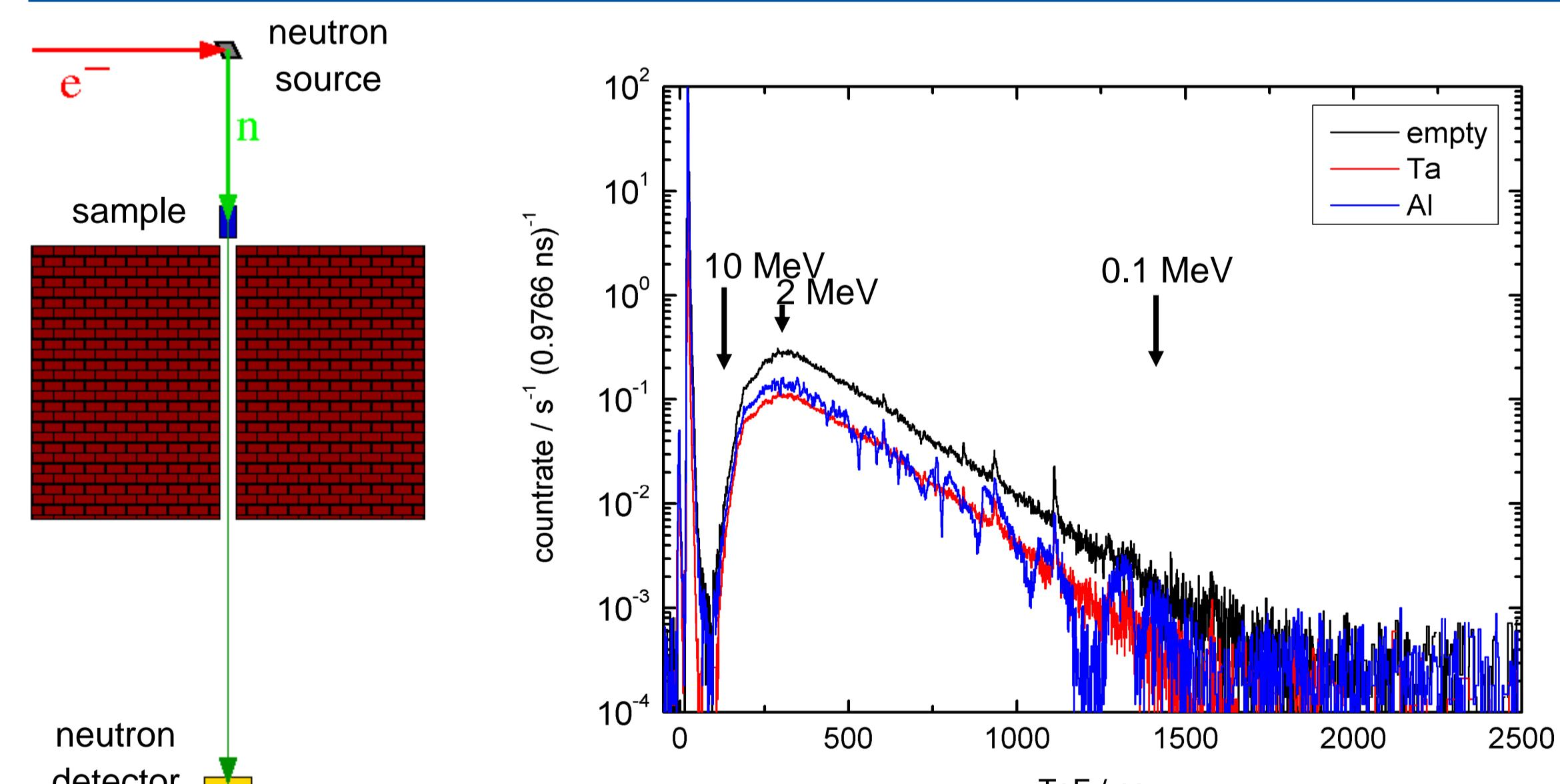
Measured neutron time-of-flight spectra with different absorbers
