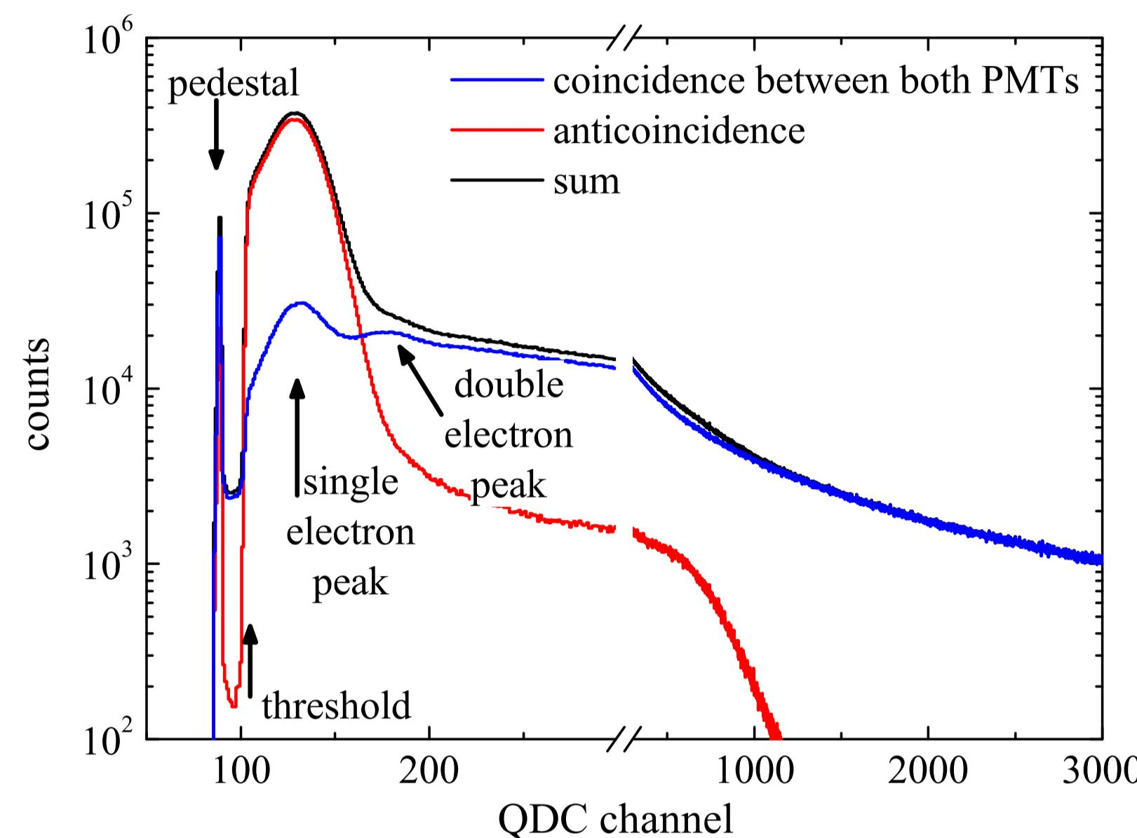
QDC spectrum of one PMT under different conditions concerning the other PMT of the same detector illustrating the SEP and the trigger threshold.
