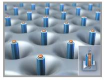
towards the edge of the nanowire; in other words, towards the surface. There, they become partially inactive and no longer contribute towards conductivity. A special method permitted the scientists to longitudinally remove the nanowires layer by layer during the measurements which, in turn, allowed them to take three-dimensional measurements. That is how they got 3D images of the conductivity inside a nanowire which only has the thickness of one 25,000th of a human hair.
