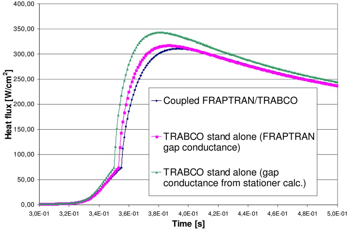
Fig. 4. Surface heat flux for the three cases, no DNB
