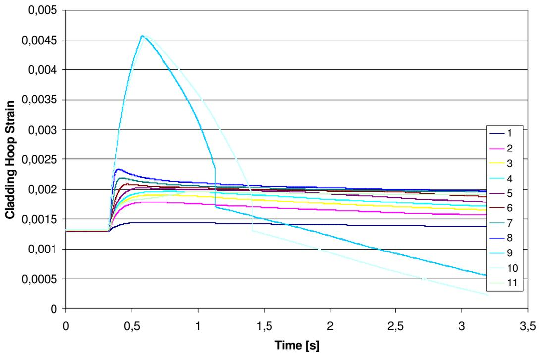
Fig. 14. Cladding hoop strain at different axial levels in case of DNB
