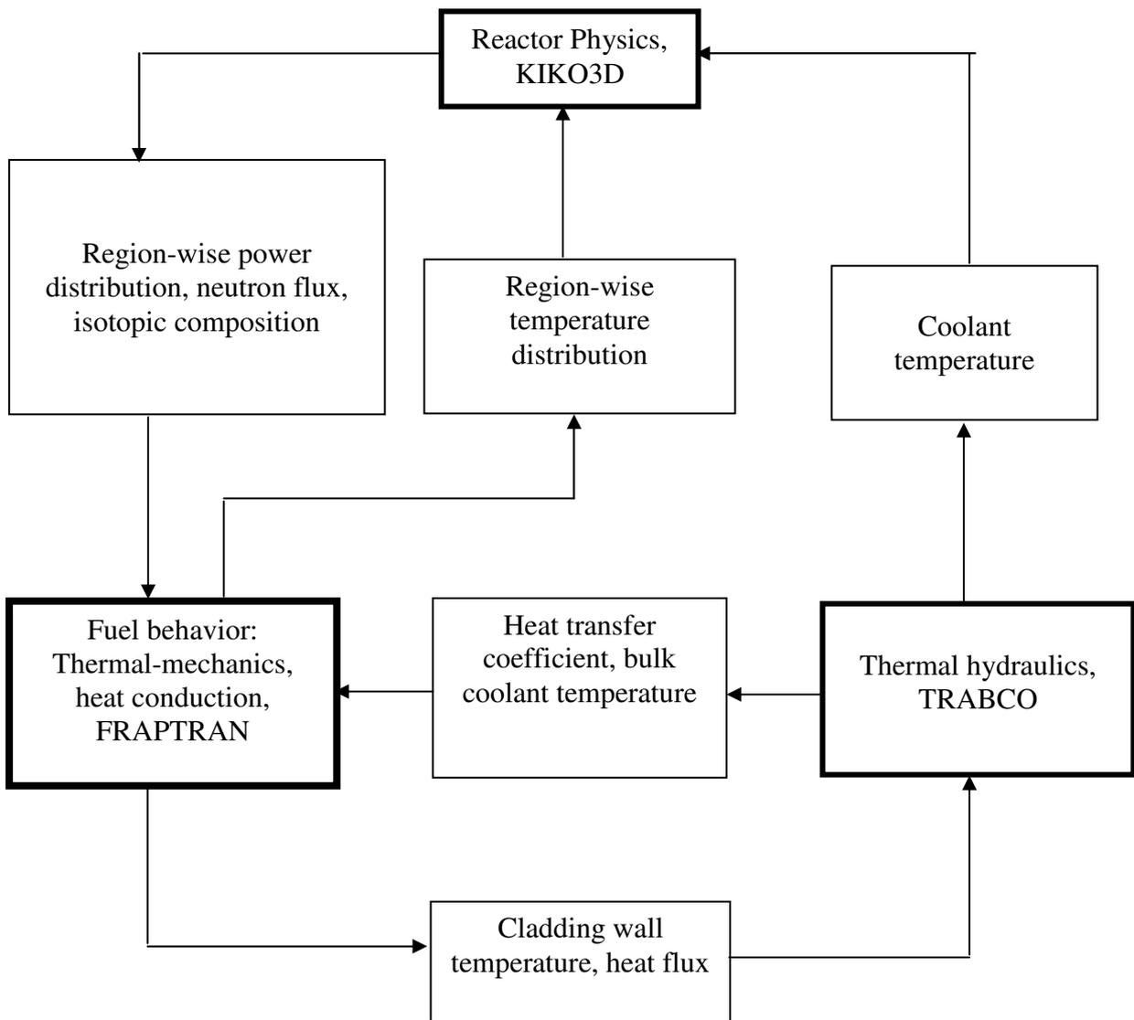
Fig. 1. The multiphysics connections between the codes representing the different disciplines
