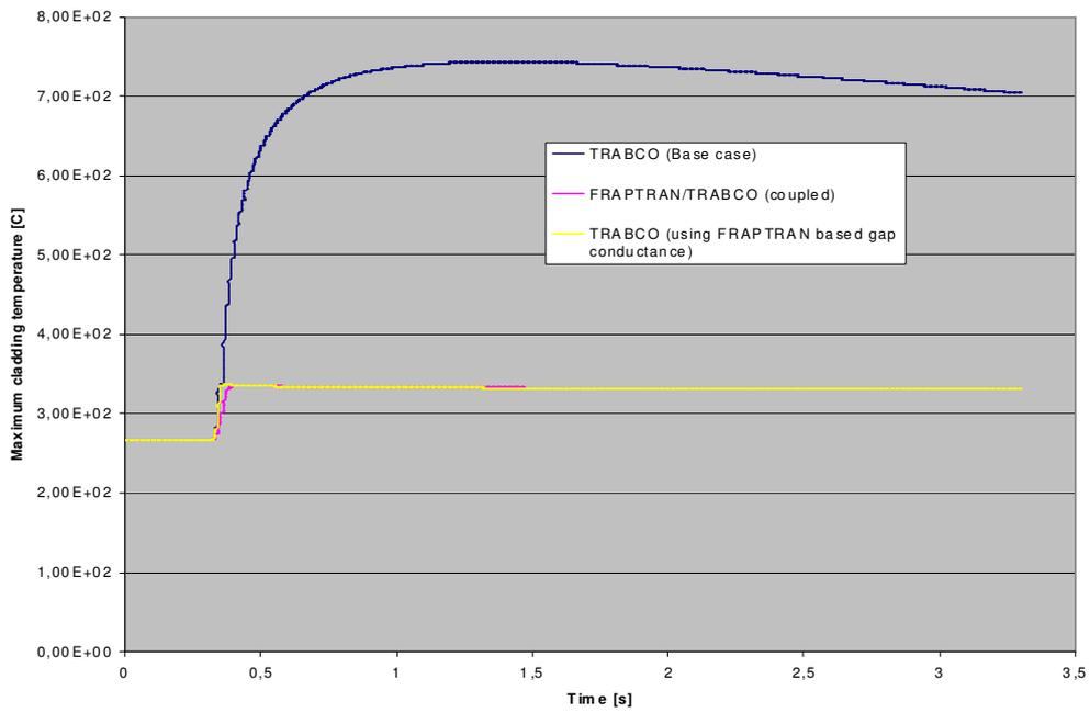
Fig. 7. Maximum cladding temperatures for the three cases, DNB in the worst case
