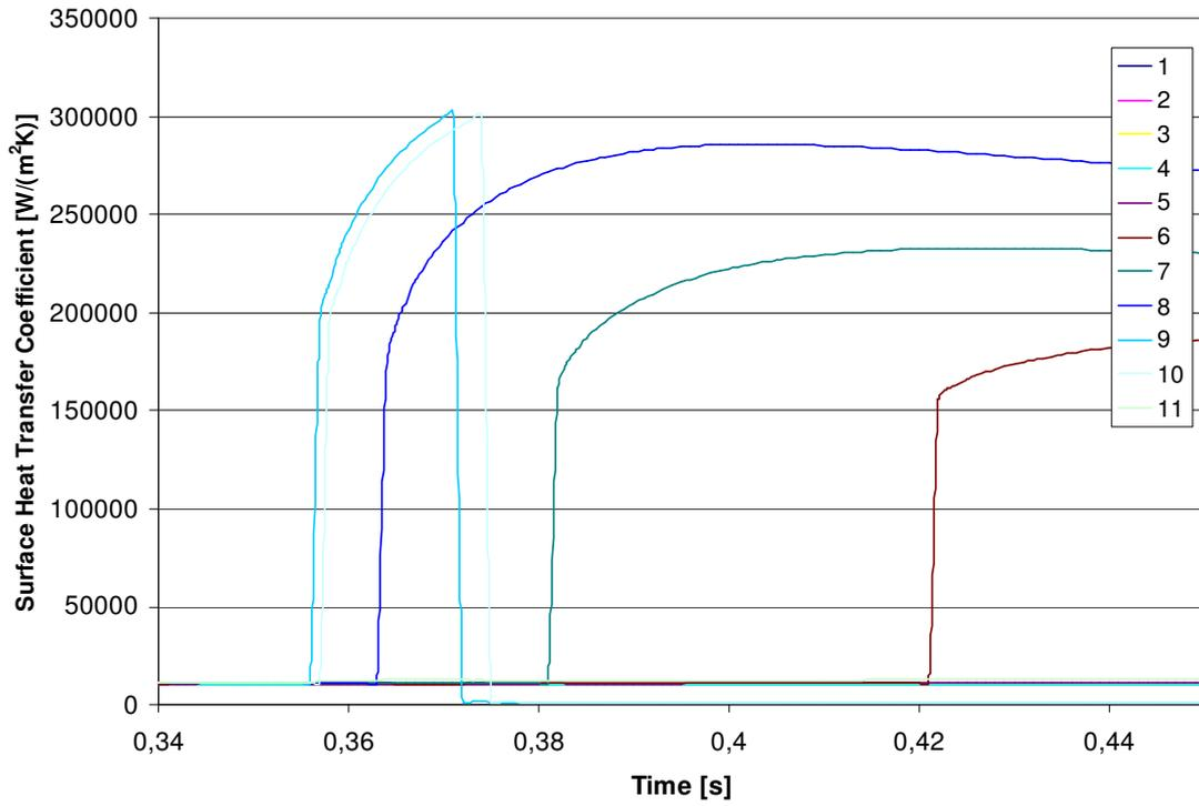
Fig. 9. Heat transfer coefficients to coolant in case of DNB
