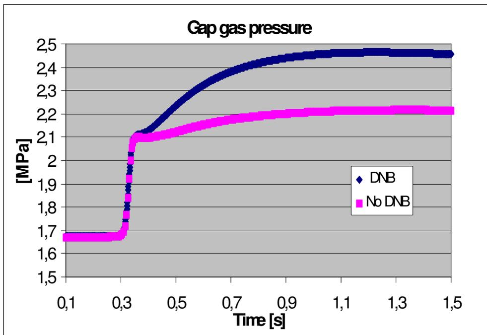
Fig. 10. Gas gap pressure
