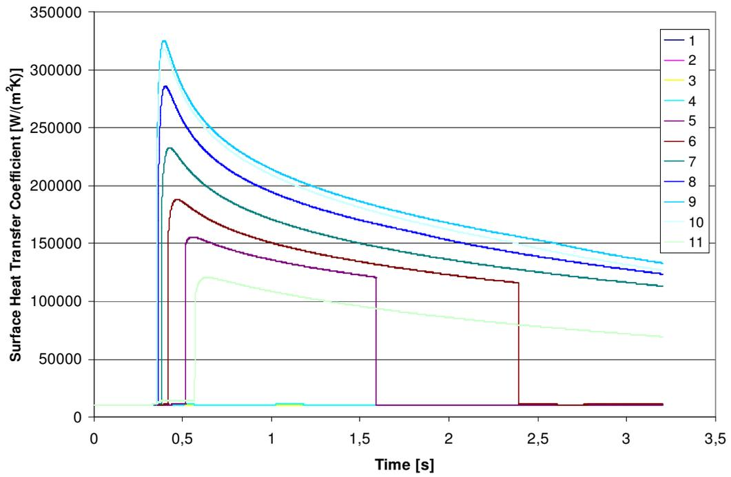
Fig. 8. Heat transfer coefficients to coolant without DNB
