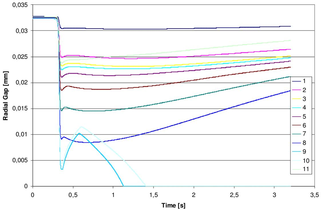
Fig. 12. Thermal mechanical processes, gap size, in case of DNB
