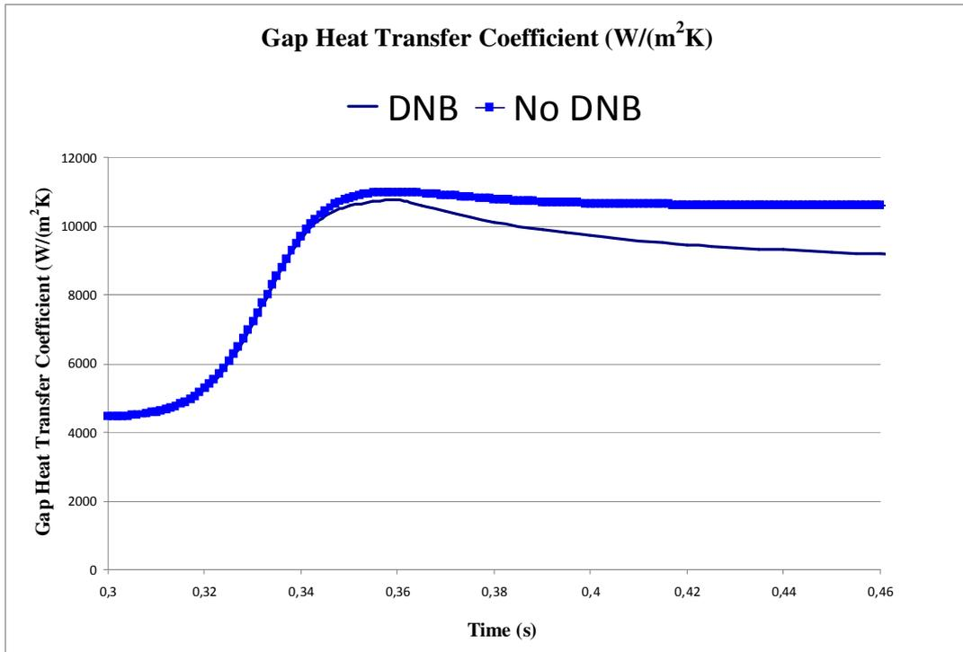
Fig. 13. Gap heat transfer coefficient
