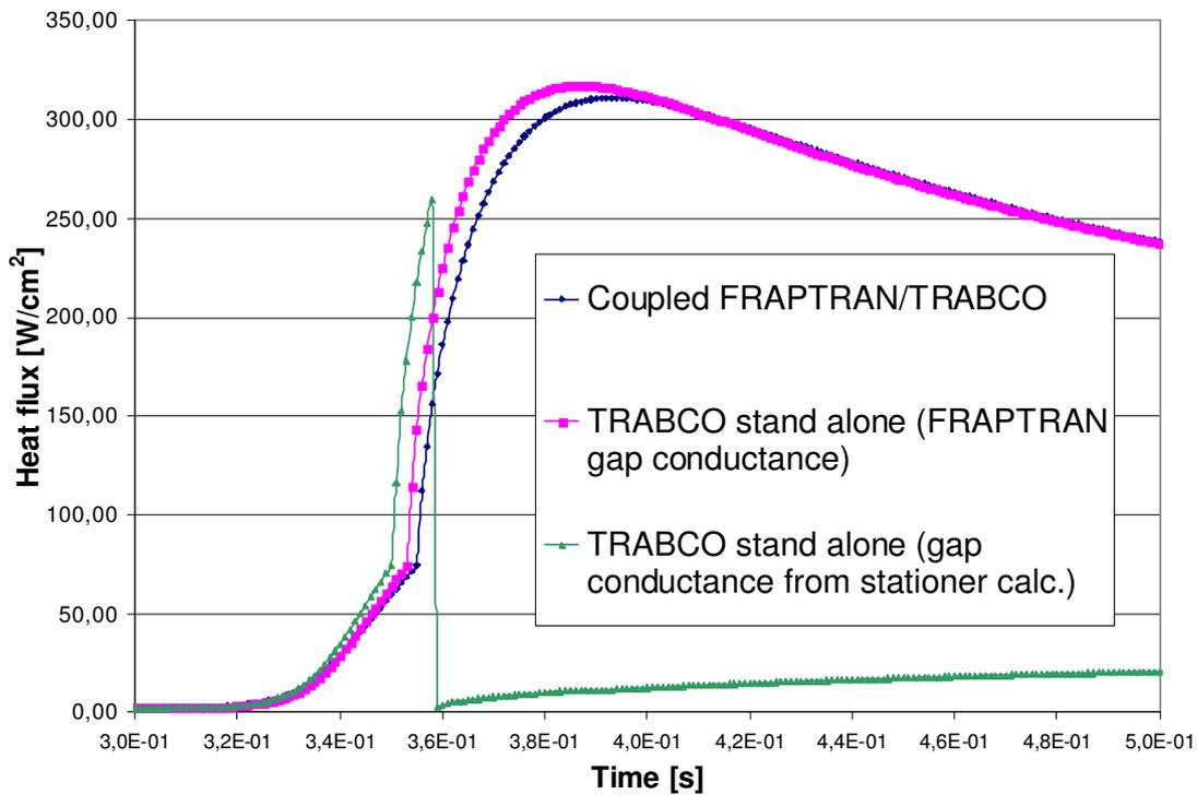
Fig. 6. Surface heat flux for the three cases, DNB in the worst case
