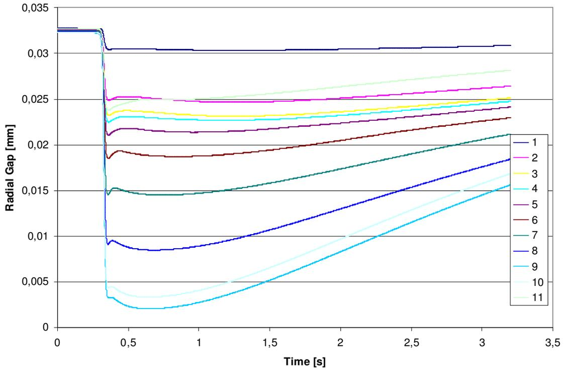
Fig. 11. Thermal mechanical processes, gap size in case of without DNB
