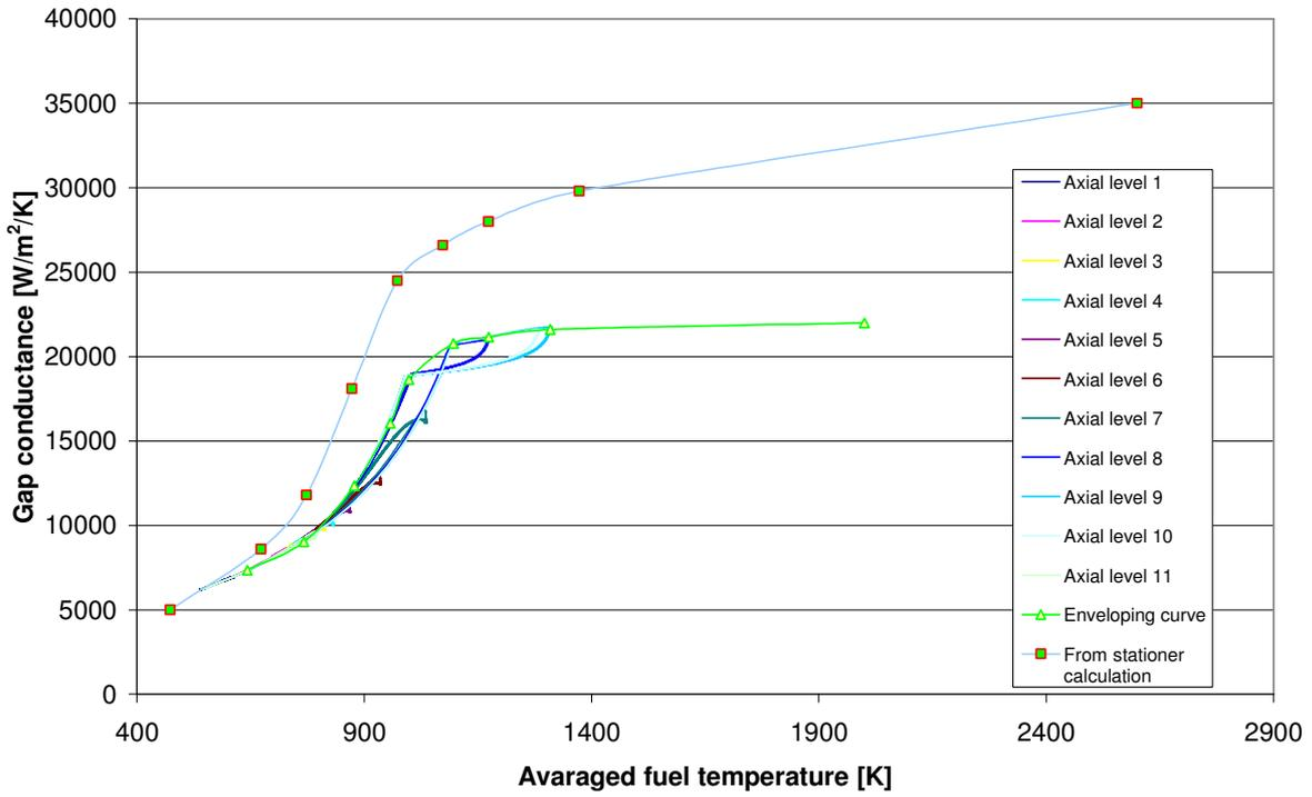
Fig. 3. Gap heat transfer coefficients from the preceding stat. calc. or from the FRAPTRAN
