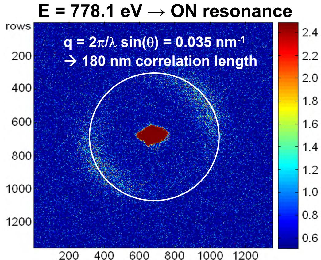
Proof-of-principle using 5th harmonic at 1.59 nm (Co L3)
