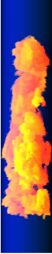
Fig. 5: Isolated large bubble in a churn-turbulent flow in the DN200 test section, J_l = 1 m/s, J_g = 1.3 m/s
