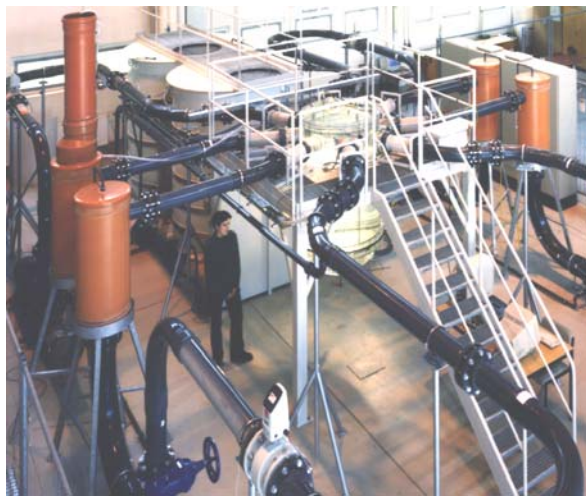
Fig. 1: View on the test facility ROCOM with the RPV model made from acryl
