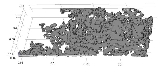
Laminar flow based model simulations (COMSOL Multiphysics) of transport in a fracture only reflects *degree of reality* of geometry extracted from CT.
