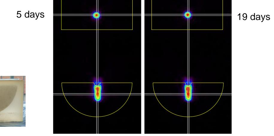
Halite half cylinder (Staßfurt), diameter 10 cm charged with 0.5 ml [<sup>124</sup>I]Q-solution: no indication for diffusional transport during observation period of 19 days - as expected for undisturbed rock salt.
