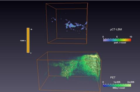
Lattice-Boltzmann-Simulation based on the µXCT-derived structural model vs. direct PET observation => General similarity in space and time, but significant discrepancies in
