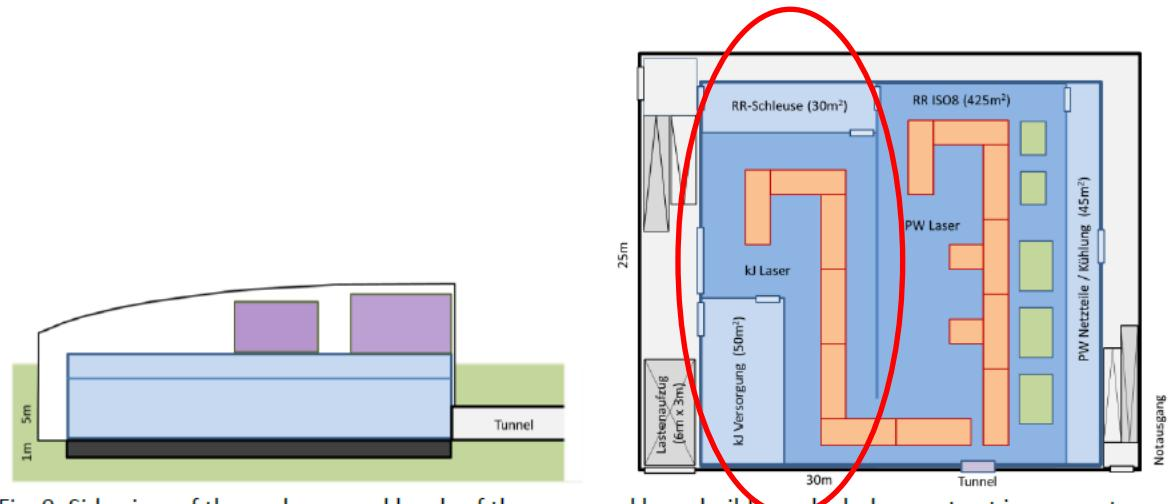
Fig. 9: Side view of the underground levels of the proposed laser building which does not yet incorporate additional office space in potential upper floors (left). Foot-print of the clean-room laser lab showing examples of PW and kJ laser table installations (right).
