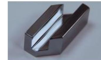
Channel-cut Si crystals:
