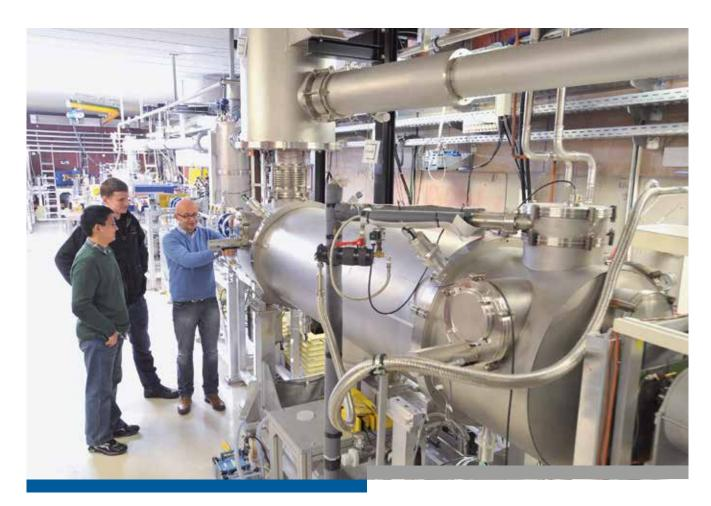
THE HEART OF THE ELBE: In an effort to enhance experimental options at the new Center for High-Power Radiation Sources, electron pulses from the electron accelerator that has been in operation for years have to be shortened and intensified by an entire order of magnitude. The electrons are used by the two free electron lasers, two new terahertz sources, as well as for the facilities for the generation of gamma and X-rays, positrons, and neutrons. Photo: Frank Bierstedt
