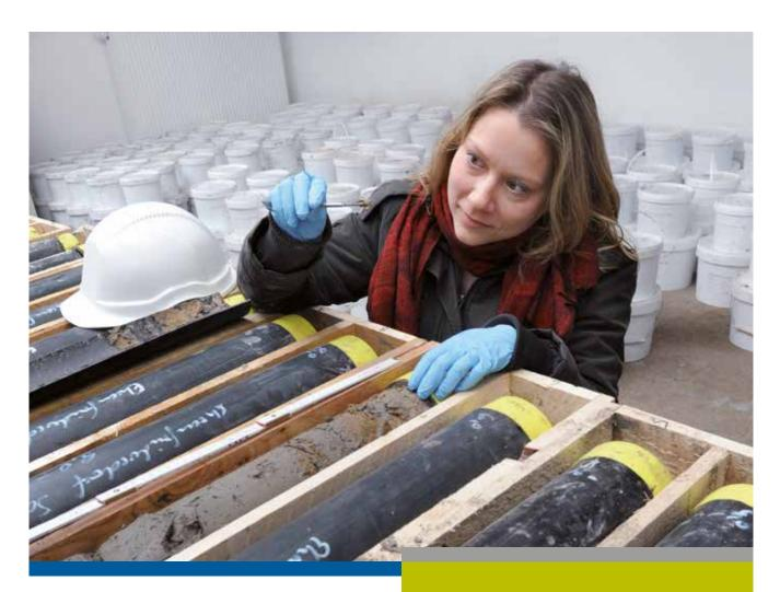
RESEARCH WORK: Before geologist Inga Osbahr is able to examine materials obtained from tailings and packaged inside PVC pipes to determine their constituent parts using an electron beam, the sandy mixture must first be prepped. Photo: VNG - Detlef Müller
