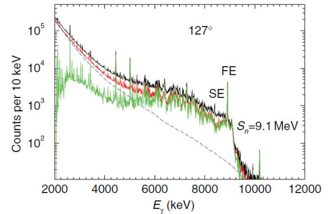
Unfolding of detector response and efficiency (GEANT4)
