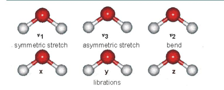
All oscillations (librations) contain Zero-point Energy NO Zero-point Energy in Free Rotations KE of each **H-atom** in Isolated H<sub>2</sub>O (Vapor phase) Exp  $v_j$  (cm<sup>-1</sup>) Vapor = 3686 3738 1596 Important: H<sub>2</sub>O Freely rotates in Vapor
