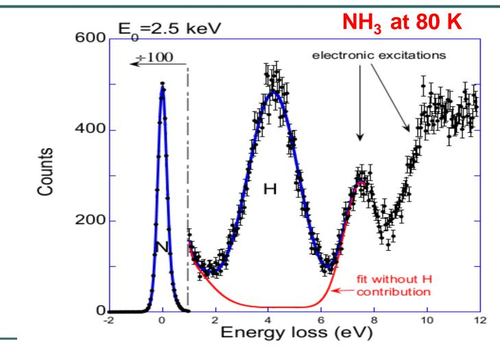
Calculated Ke(H) in NH<sub>3</sub> (note continuity S-L-Gas) Major part of Ke(H) is ZP motion 148 meV vs 150 meV (vapor) Prelim ECS (Vos Exp) :  $149 \pm 7$  meV
