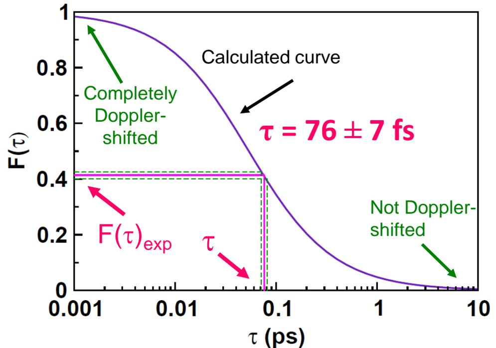
$$E_\gamma(\theta) = E_\gamma \left[ 1 + F_{\text{exp}}(\tau) \frac{V_{\text{cm}}}{c} \cos \theta \right]$$
