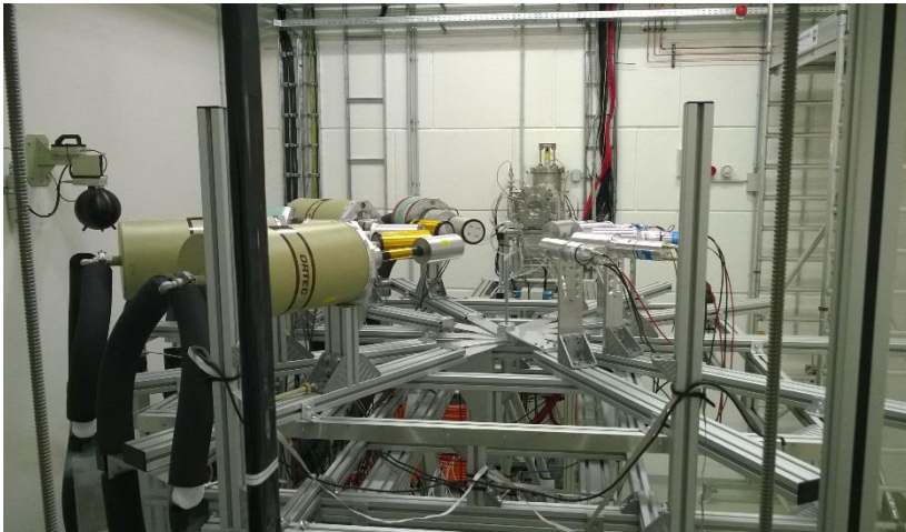
HPGe + LaBr 3 for angular distributions and inelastic neutron scattering
