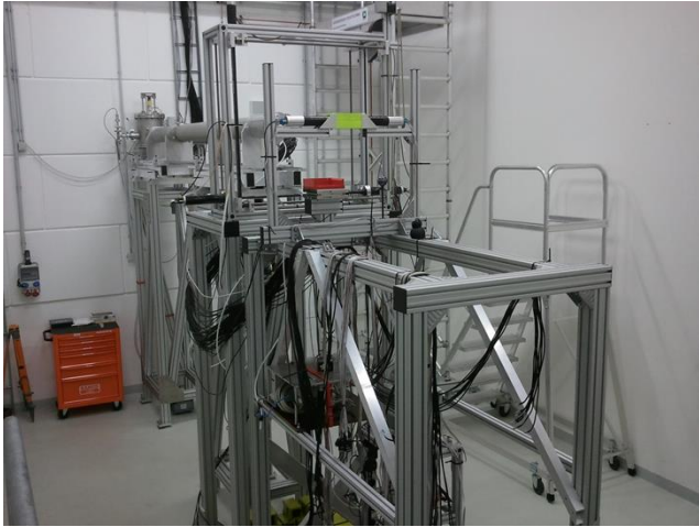
Transmission set-up for total cross sections
