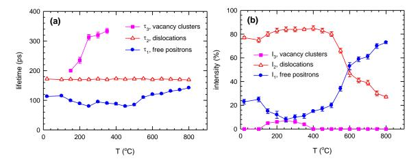
Fig. 1: Results of positron lifetime investigations of hydrogen loaded Ti (H<sub>2</sub> gas pressure 1 bar, temperature 400 °C): the development of (a) positron lifetimes and (b) corresponding relative intensities on the annealing temperature.
