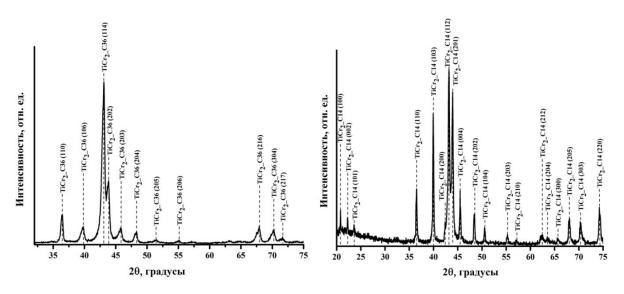
Fig1. Diffractograms of TiCr2 alloys obtained in an anomalous glow discharge plasma (a) and electron-beam melting (b)
