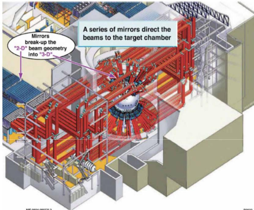
NIF Laser System: 192 laser beams
