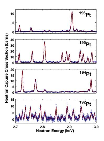
$$A_{\gamma} = g\Gamma_{n}\Gamma_{\gamma}/(\Gamma_{n}+\Gamma_{\gamma})$$
