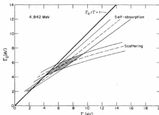
FIG. 7. Combined results of the self-absorption and scattering measurements for the 4.842 MeV level in  $^{208}\text{Pb}$ . The dashed curves indicate combinations of  $\Gamma_0$  and  $\Gamma$  which reproduce the experimental results; the solid curves represent the error band for each case. The shaded region contains the values of  $\Gamma_0$  and  $\Gamma$  consistent with both experiments, and with the condition  $\Gamma_0/\Gamma \leq 1$ .
