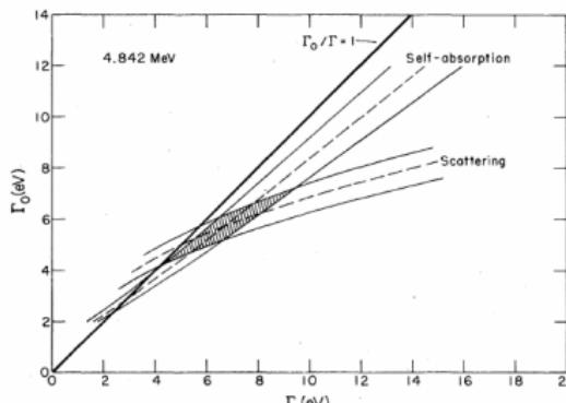
FIG. 7. Combined results of the self-absorption and scattering measurements for the 4.842 MeV level in  $^{208}\text{Pb}$ . The dashed curves indicate combinations of  $\Gamma_0$  and  $\Gamma$  which reproduce the experimental results; the solid curves represent the error band for each case. The shaded region contains the values of  $\Gamma_0$  and  $\Gamma$  consistent with both experiments, and with the condition  $\Gamma_0/\Gamma \leq 1$ .
