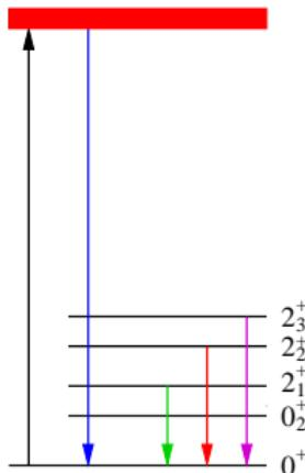
Filled circles:  $B_0 = \frac{I_{\text{g.s.}}}{I_{\text{g.s.}} + I_{2_1^+} + I_{2_2^+} + I_{2_3^+}}$
