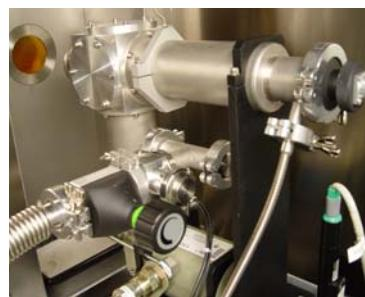
**Closed-cycle He cryostat** with large fluorescence window adapted to the 13-element detector and very low vibration levels cools samples down to 15 K.
