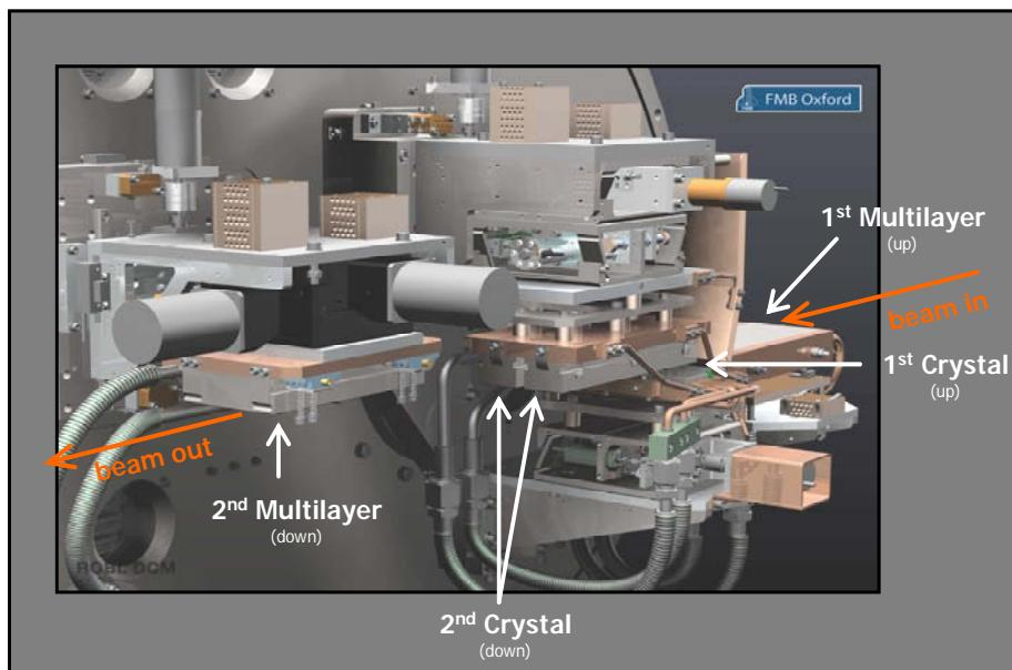
**Fig. 4.** Design drawing of the combined double crystal/double multilayer monochromator. The 1<sup>st</sup> multilayers are mounted together with the 1<sup>st</sup> and 2<sup>nd</sup> crystals on a common Bragg drive, while the 2<sup>nd</sup> multilayers are mounted on an independent stage.
