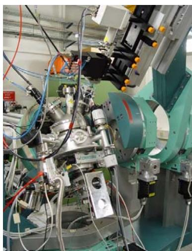
Fig. 1.: Sputter deposition chamber.
