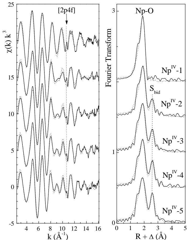
**Fig. 3.** Np L<sub>3</sub>-edge  $k^3$ -weighted EXAFS spectra (left), and the corresponding Fourier transforms (right) of Np(IV) sulfate species.
