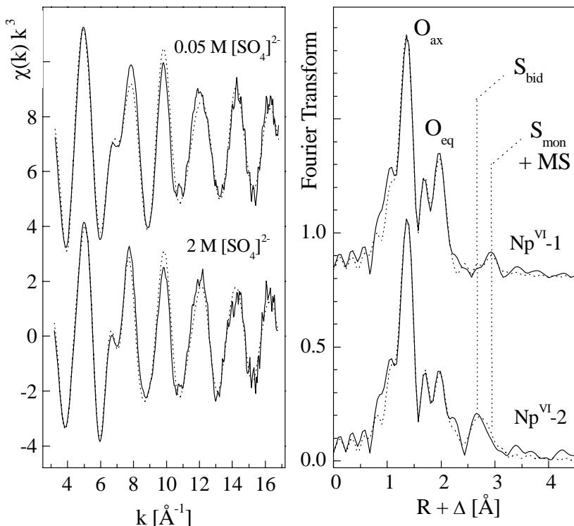
**Fig. 1.** Np L<sub>3</sub>-edge  $k^3$ -weighted EXAFS spectra (left), and the corresponding Fourier transforms (right) of Np(VI) sulfate species.
