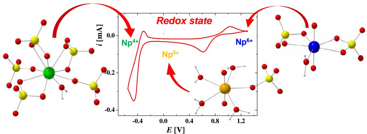
**Fig. 4.** Cyclic voltammograms of 0.05 M Np(VI) in an aqueous solution of 2.0 M  $(\text{NH}_4)_2\text{SO}_4$  at pH 1.1, Au working electrode, start potential 1.3 V, initial scan direction: cathodic, scan rate: 400 mV/s. The sulfate coordination of the  $\text{Np}^{4+}$ ,  $\text{Np}^{5+}$  and  $\text{Np}^{6+}$  solution species is shown as schematic structure drawing.
