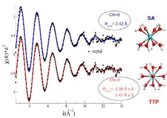
**Fig. 1.** Experimental (black points) and fitted (SA (CN=8) red and TTP(CN=9) blue lines) Cf L<sub>III</sub>-edge EXAFS spectrum of Cf<sup>III</sup>-aq.
