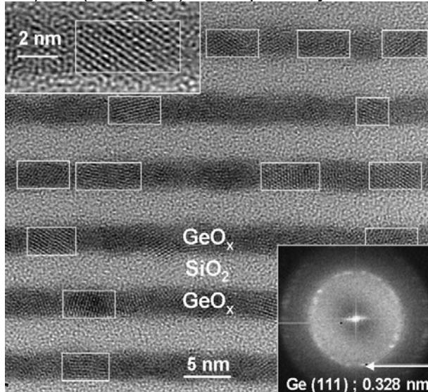
For sample #SL-02 crystallisation is starting also slightly above  $500^\circ\text{C}$ . After  $T_A = 630^\circ\text{C}$  annealing the NC size of 4.7 nm corresponds with the  $\text{GeO}_x$  sublayer thick-
