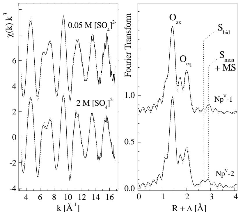
**Fig. 2.** Np  $\text{L}_3$ -edge  $k^3$ -weighted EXAFS spectra (left), and the corresponding Fourier transforms (right) of  $\text{Np(V)}$  sulfate species.
