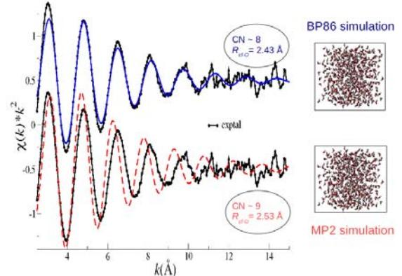
**Fig. 2.** Comparison of the  $k^2$ -weighted Cf-L<sub>III</sub> edge EXAFS spectrum of Cf<sup>III</sup>-aq (black points) with the simulated spectra obtained from the MC BP86 (blue line) or MP2 (red line) simulation.
