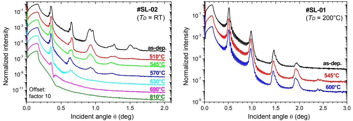
**Fig. 2:** XRR of #SL-02 ( $T_D = \text{RT}$ ) measured after deposition and during post-annealing treatment up to 690°C.
