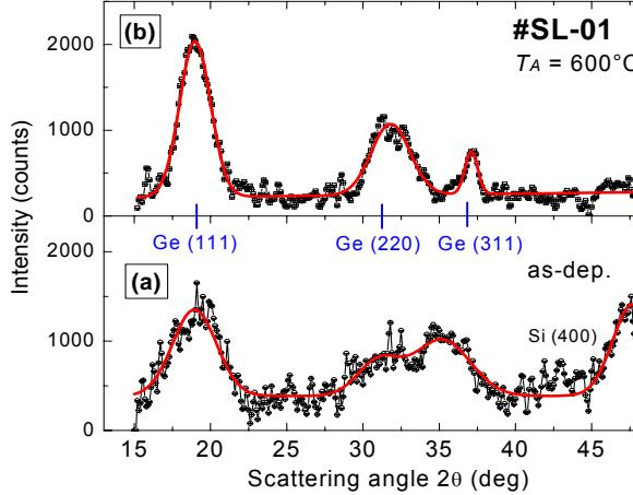
**Fig. 4:** GIXRD ( $\alpha_i = 0.25^\circ$ ) for #SL-01 ( $T_D = 200^\circ\text{C}$ ). (a) As-deposited pattern with the glassy near-order peak of Ge. (b) XRD pattern obtained after annealing at  $600^\circ\text{C}$ . From (111) and (220) Ge reflections an average NC size of  $(2.6 \pm 0.2)$  nm can be derived.
