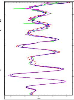
**Figure 2.** Overlay of the U L<sub>III</sub>-edge EXAFS spectra of uranium(VI)-desferrioxamine B solutions recorded at three different pH values with that corresponding to an acidic  $\text{UO}_2(\text{NO}_3)_2$  solution (red).
