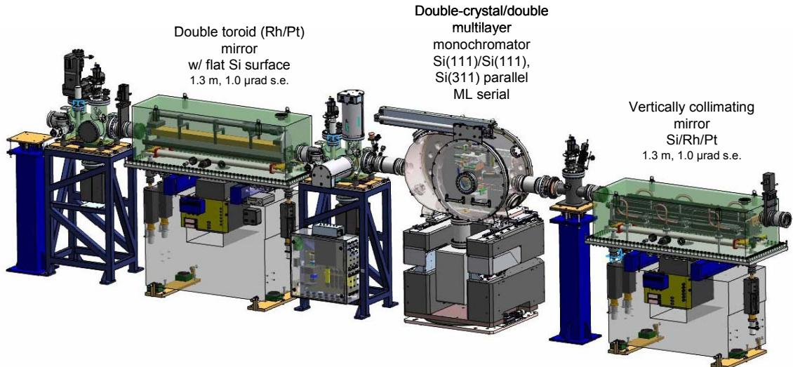
**Fig. 2.** Design drawing of new optical components.
