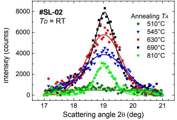
**Fig. 5:** #SL-02 ( $T_D = 25^\circ\text{C}$ ): Development of Ge(111) bragg peak intensity during annealing. The loss in intensity at  $T_A = 810^\circ\text{C}$  indicates a strong loss of Ge (60%), while the Ge NC are even bigger then at  $T_A = 690^\circ\text{C}$ . The lines represent the fitting results.
