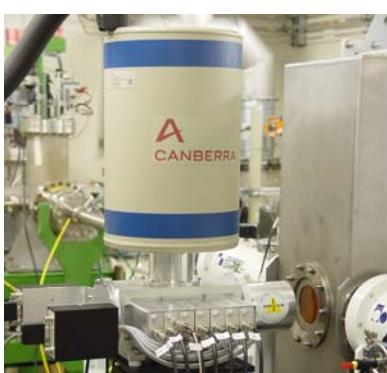
**13 element LEGe detector** with a high-rate digital multi-channel analysis spectrometer (XIA) and dedicated analysis program integrated into the XAS data collection software XATROS.
