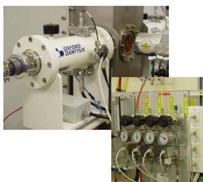
**3-kV ionization chambers** with remote-controlled gas mass-flow controllers.
