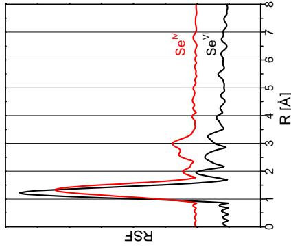
Fig. 1. Fourier transforms of Se(VI) (black) and Se(IV) (red) sorbed onto anatase at pH 3.5.
