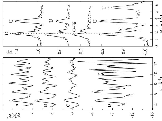
Fig. 1. Uranium L<sub>3</sub> edge EXAFS (left) and their corresponding Fourier transform (right) of UO<sub>n</sub>(OH)<sub>4.2n</sub>mH<sub>2</sub>O colloid (sample **A**), colloid samples with initial molar Si:U ratios of 0.83 (sample **B**) and 1.68 (sample **C**), and synthetic coiffinite (sample **D**); the spectrum of sample **D** was collected at 15 K, the measurement of the other samples was performed at room temperature.
