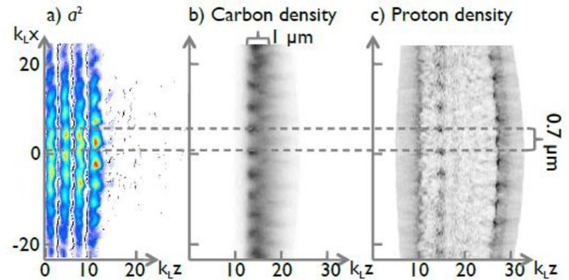
FIG. 4. (colour online) Simulation snap-shots of a) laser intensity,  $\langle a^2 \rangle$ ; b) carbon ion density; and c) proton density for a simulation with  $d = 10$  nm (312 fs after the pulse first reaches the target).
