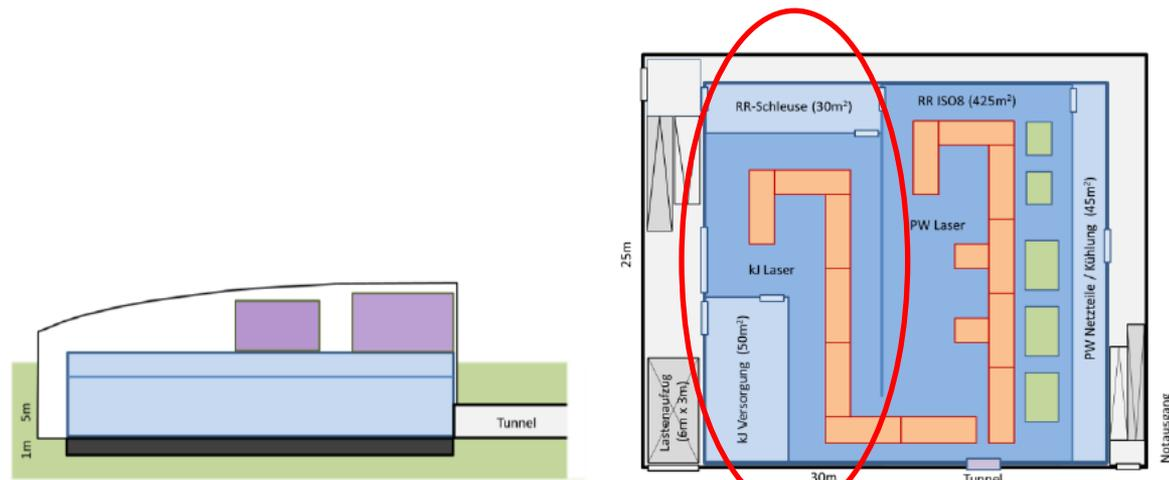
Fig. 9: Side view of the underground levels of the proposed laser building which does not yet incorporate additional office space in potential upper floors (left). Foot-print of the clean-room laser lab showing examples of PW and kJ laser table installations (right).
