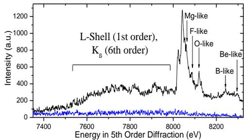
Self emission spectroscopy  $\Delta t \sim 5-10$  ps
