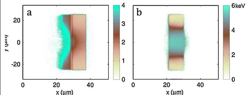
Self-generated magnetic confinement of hot electrons and enhanced heating
