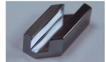
Channel-cut Si crystals:
