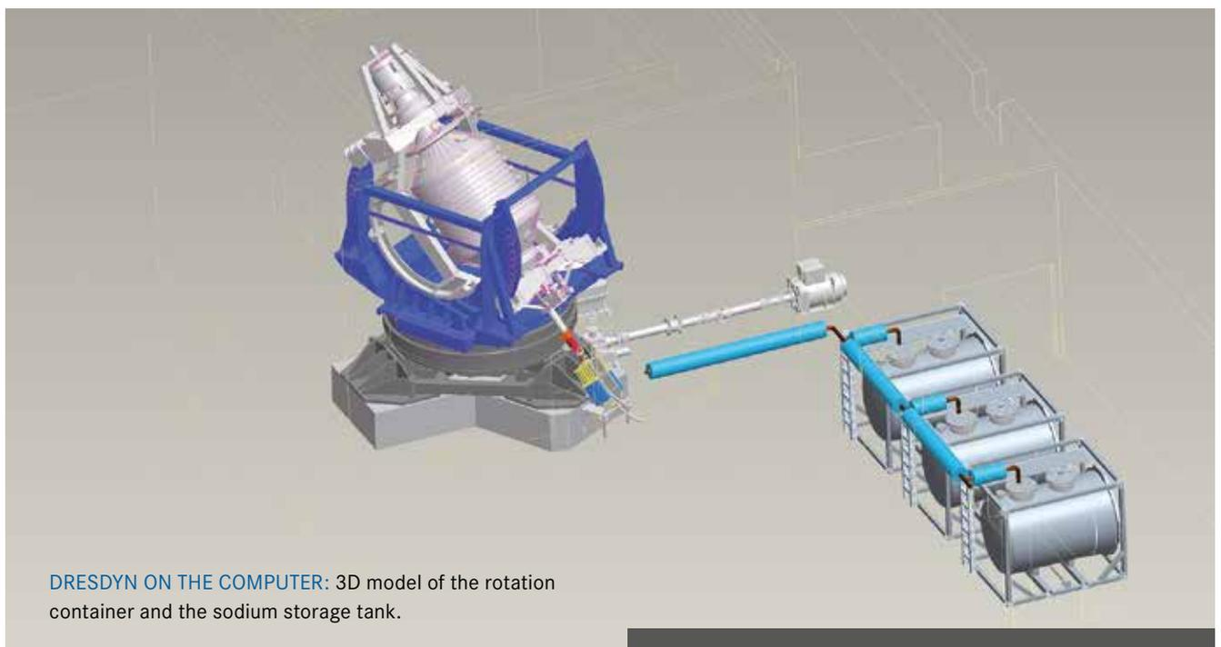
**DRESDYN ON THE COMPUTER:** 3D model of the rotation container and the sodium storage tank.
