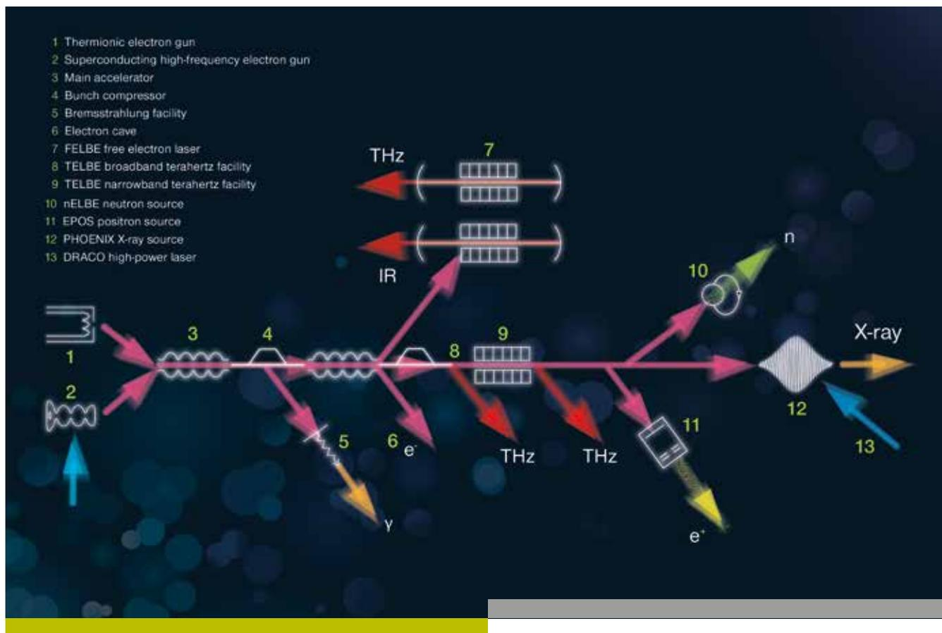
**UNIVERSAL DEVICE:** Electrons | pink | from the ELBE particle accelerator are converted into light in the infrared and terahertz range | red |, into X- and gamma rays | orange | and into neutrons | green | and positrons | yellow |. The PHOENIX facility for extremely short-wave and intense X-ray light (12) is one of the latest developments at the ELBE. X-rays are produced by coupling electrons and light | blue | from a high-power laser.
