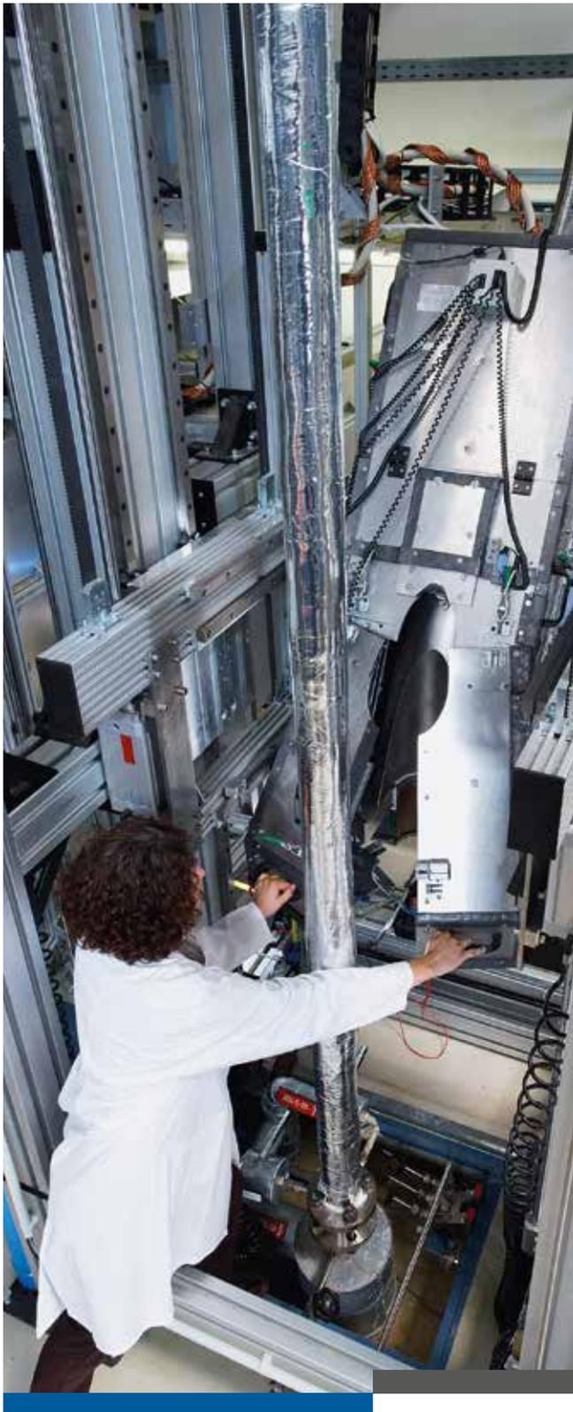
**RAPID IMAGES:** Electrical engineer Martina Bieberle is using images of liquid and gas flow mixtures taken with X-ray tomograph ROFEX. What makes them stand out is their unusually high temporal resolution. Photo: Rainer Weisflog
