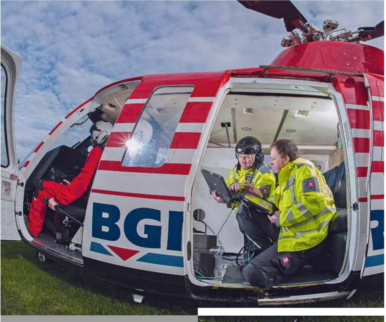
**MEASURING FLIGHT:** This helicopter is capable of detecting raw materials that are hidden up to 500 meters below the surface.
