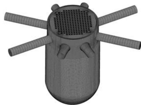
Fig. 3: Outline of the ROCOM ANSYS-CFX calculation grid.
