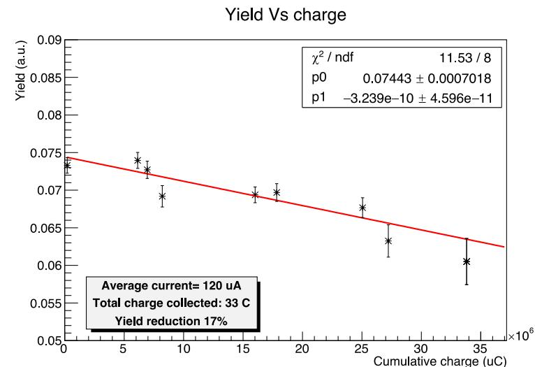
Good target stability with high current intensity proton beam @ LUNA (120  $\mu\text{A}$ )
