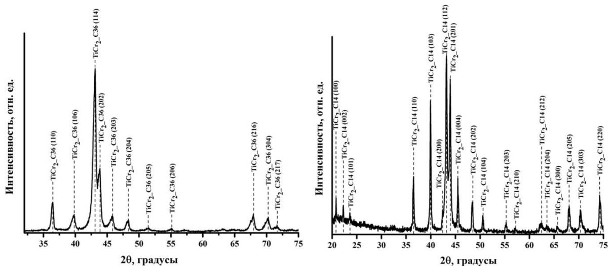
Fig1. Diffractograms of TiCr<sub>2</sub> alloys obtained in an anomalous glow discharge plasma (a) and electron-beam melting (b)
