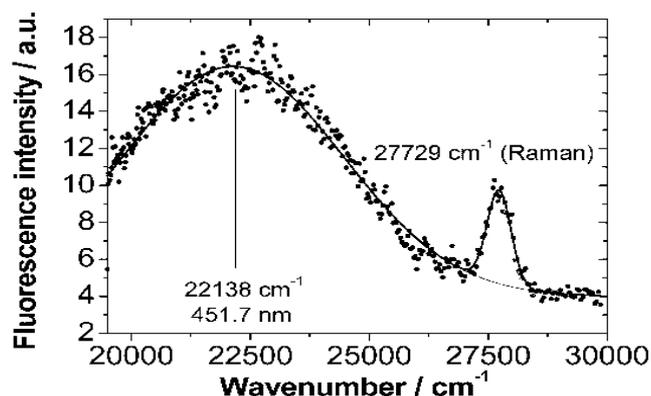
Fig. 1: Fluorescence spectrum of 2,3-dihydroxybenzoic acid in 1 M HClO<sub>4</sub>
