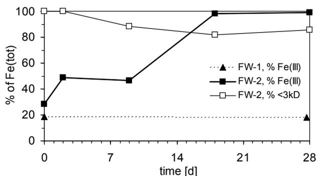
Fig. 1: Percentages of Fe(III) and <3kD fraction based on Fe(tot) concentration in the water samples FW-1 and FW-2 over time.
