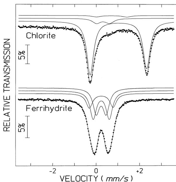
Fig. 1: Moessbauer spectra of pure chlorite and pure ferrihydrite.
