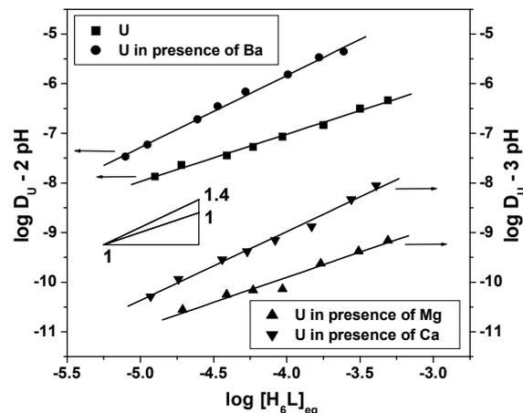
Fig. 2: Uranium extraction by  $LH_6$  in absence and presence of competing ions at  $pH_{0.5}$  as a function of ligand concentration. Organic phase:  $[LH_6] = 1.3 \times 10^{-5}$  to  $5 \times 10^{-4}$  M,  $CH_2Cl_2$ . (Due to different pH and pH-dependencies the order seen in Fig. 1 is not reflected here.)
