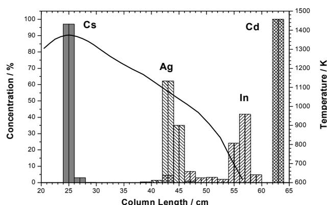
Fig. 1: The deposition of Ag, Cd, In and Cs on quartz surfaces.
