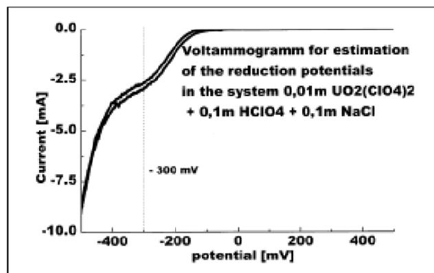
Fig.2: Current-potential curve for estimation of the reduction potential for uranium
