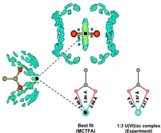
Fig. 2: MCTFA result. Brighter balls indicate U positions with the highest likelihood (good fits), darker balls indicate positions resulting in poorer fits. U-atom bond distances are given for the optimum position (black dots).
