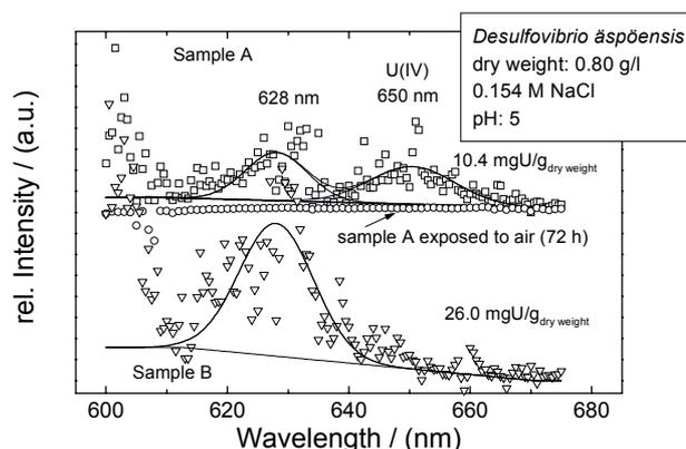
Fig. 1: LIPAS spectra of uranium in suspensions of *D. äspöensis*.
