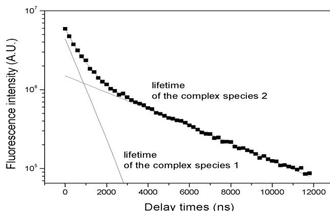
Fig. 2: Bi-exponential fluorescence decay of the solution with  $5 \cdot 10^{-5}$  M uranium and  $1.25 \cdot 10^{-4}$  M p-threonine (1:2.5) at pH 4
