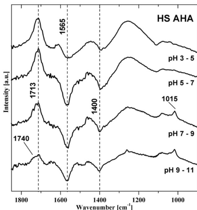
Fig. 1: pH induced FT-IR difference spectra of AHA dissolved in H<sub>2</sub>O. The pH change is given in the figure.
