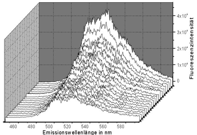
Fig. 2: TRLFS measurements of uranium(VI) sorbed onto muscovite crystals
