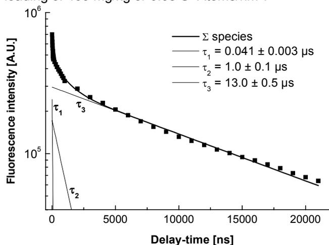
Fig. 1: Fluorescence decay of uranium(VI) sorbed on pyrophyllite at pH 5.8
