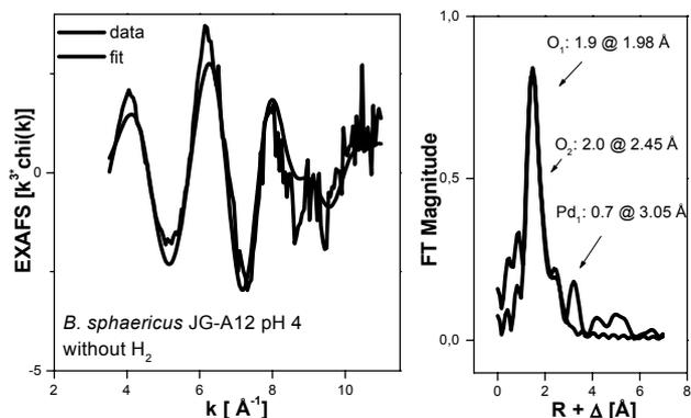
Fig. 2: Pd K-edge EXAFS spectra and their corresponding FT of the Pd nanoclusters formed at the cells of *B. sphaericus* JG-A12 at pH 2 and 4 in the absence of  $\text{H}_2$ .
