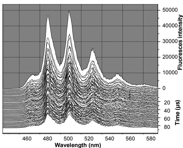
Fig. 2: Fluorescence spectra of synthetic swartzite as a function of delay time
