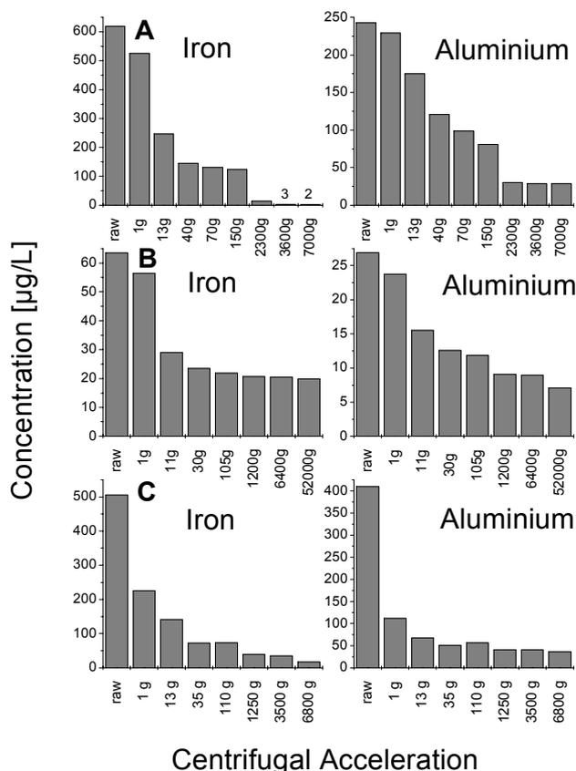
Fig.1: Al and Fe concentration after 1-hour centrifugations at various centrifugal accelerations in the water of the “Rothschönberger Stolln” adit (A), the Kaitzbach creek (B) and the river Elbe (C)
