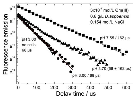
Fig. 3: Fluorescence lifetimes in the system Cm(III) - *D. äspöensis*; mono- and bi-exponential decay behavior.
