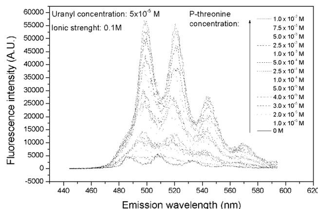
Fig. 1: Fluorescence spectra of uranium (VI) as function of the O-Phospho-L-threonine concentration at pH 4
