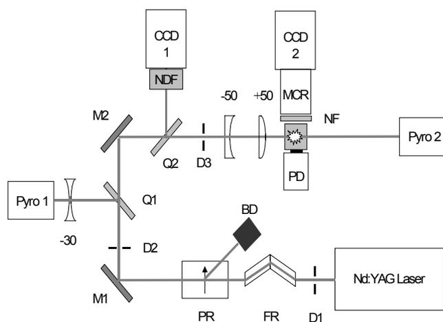
Fig. 1: Optics system of the experimental set-up. For details see text.
