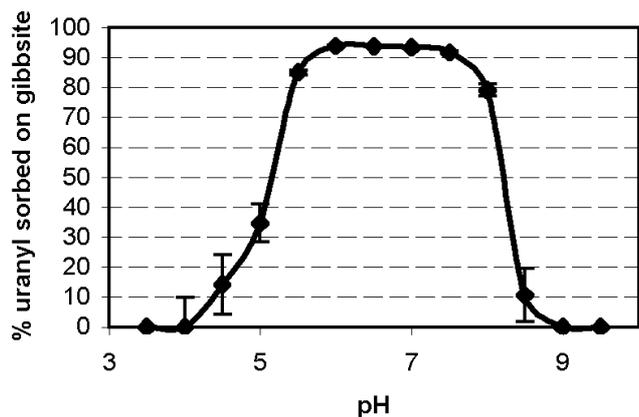
Fig. 1: Uranium sorbed on gibbsite in dependence on pH-value (Batch Experiments)
