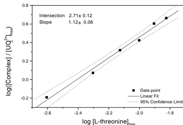
Fig. 3: Slope analysis of the complex formation at pH 4 and ionic strength of 0.1 M
