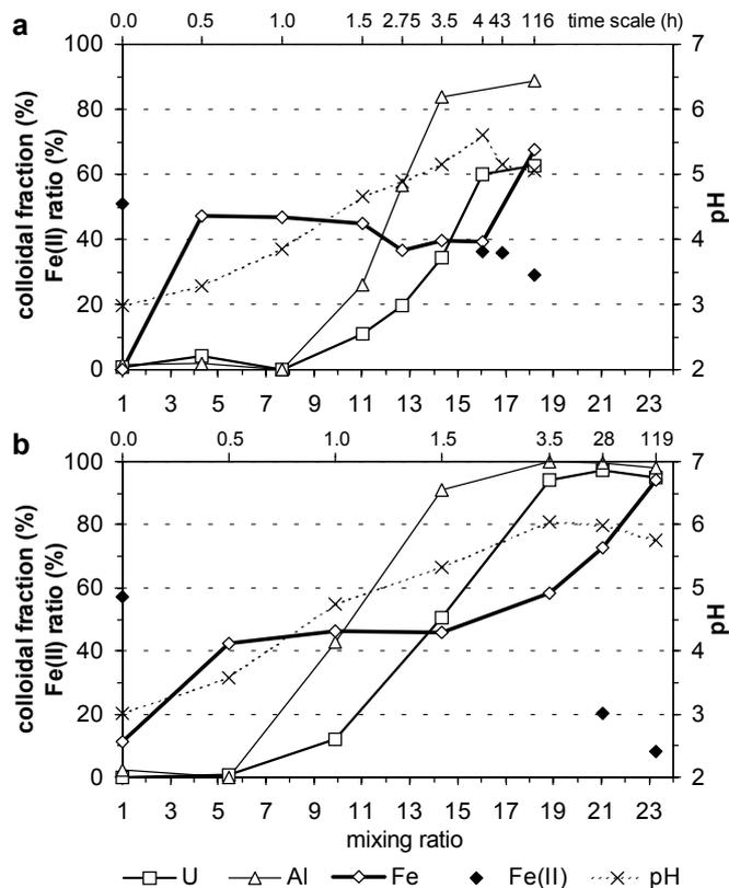
Fig. 1: Percentages of colloidal U, Al, Fe, and Fe(II) fraction (left ordinate) and pH (right ordinate) depending on mixing ratio (lower abscissa) and course of time (upper nonlinear abscissa) in the two batches of acid floodwater mixed by oxic groundwater up to a final pH 5.0-5.5 (a) and 5.5-6.0 (b). The colloidal metals were identified by 3 kD ultrafiltration.
