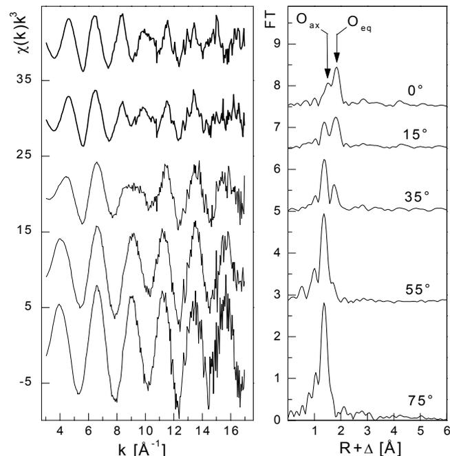
Fig. 1: U L<sub>1</sub>-edge EXAFS spectra and their Fourier transforms at different angles  $\alpha$ .
