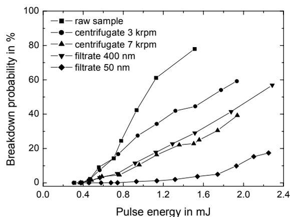
Fig. 2: Breakdown probability vs. pulse energy for various fractions of Kaitzbach source water
