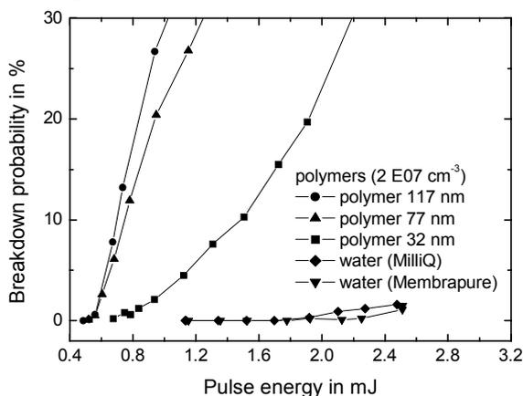
Fig. 1: Calibration using various polymer standards, background of two deionized waters
