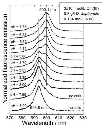
Fig. 1: Fluorescence emission spectra of Cm(III) in a suspension of *D. äspöensis* at different pH.
