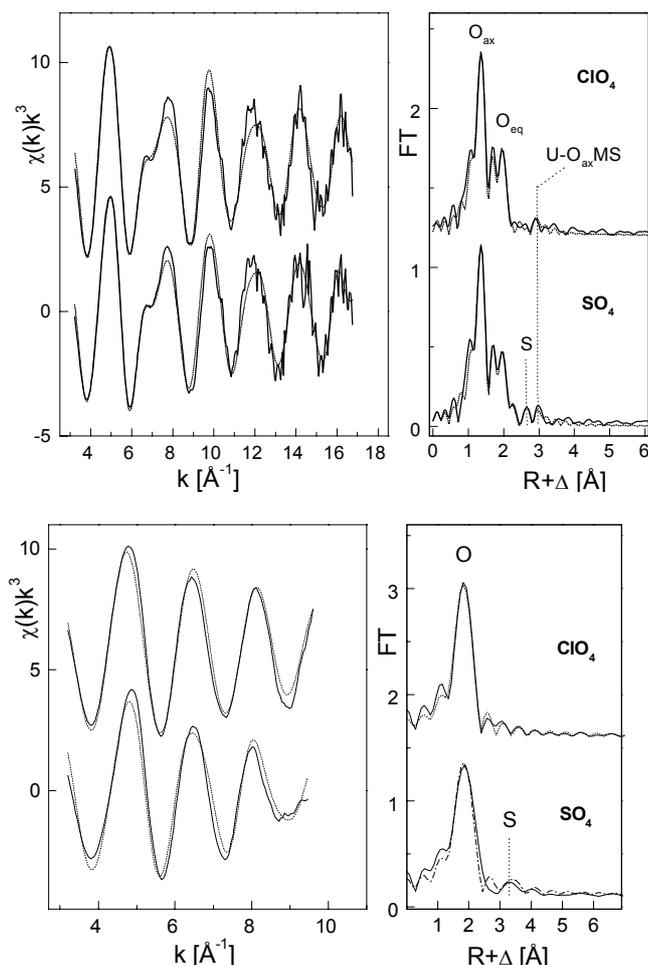
Fig. 1: U L<sub>III</sub>-edge EXAFS spectra and their Fourier transforms before (top) and after (bottom) reduction
