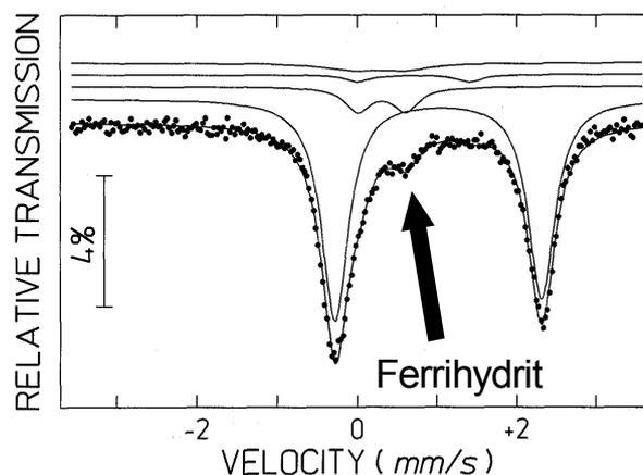
Fig. 2: Moessbauer spectrum of a chlorite sample obtained from a mixed-flow reactor experiment.
