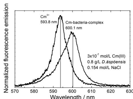
Fig. 2: Spectra of the single components of Cm(III) in suspensions of *D. äspöensis*.
