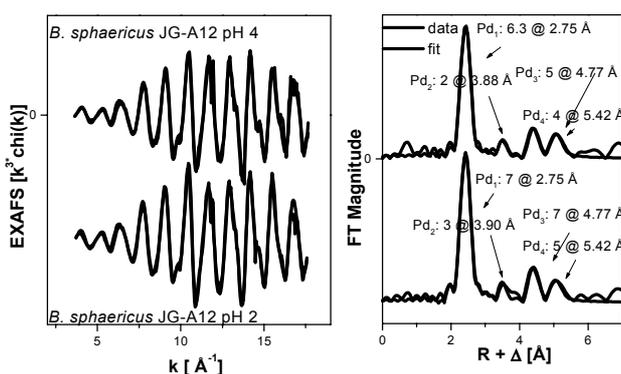
Fig. 1: Pd K-edge EXAFS spectra and their corresponding FT of the Pd nanoclusters formed at the cells of *B. sphaericus* JG-A12 at pH 2 and 4 in the presence of  $\text{H}_2$ .
