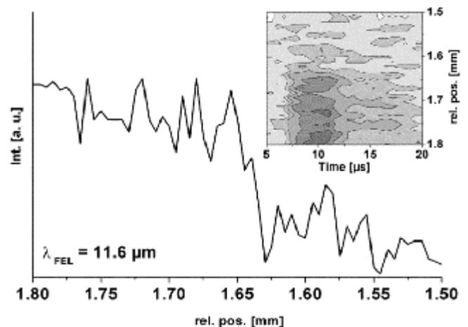
Fig. 2: Absorption profile of the border range between  $\text{O}^+$ -doped and pure germanium (extracted from inset;  $t = 10.6 \mu\text{s}$ ). Inset: mapping plot of the set of time curves of the deflection signal.
