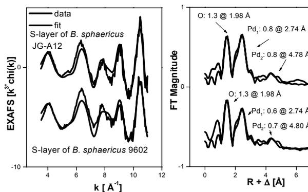
Fig. 3: Pd K-edge EXAFS spectra and their corresponding FT of the Pd nanoclusters formed at the S-layer of *B. sphaericus* JG-A12 and 9602.
