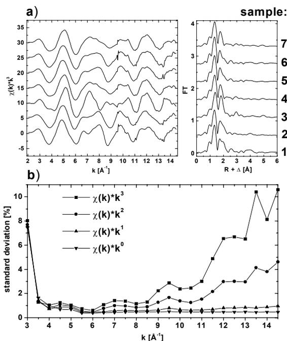
Fig. 1: a) EXAFS spectra and Fourier transforms of model compounds (1-3) and their mixtures (4-7). b) Error of relative concentrations as a function of k-ranges and k-weightings.
