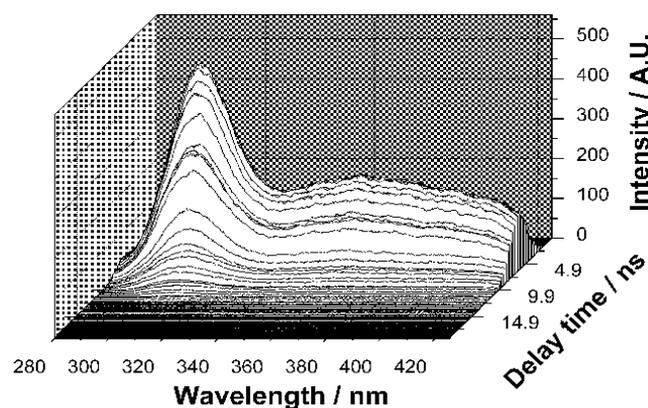
Fig. 4: Fluorescence of uranium(IV) in phosphoric acid
