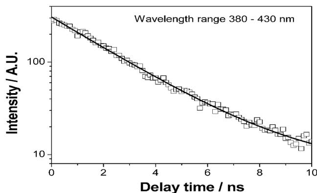
Fig. 3: Fluorescence decay of uranium(IV) in perchloric acid
