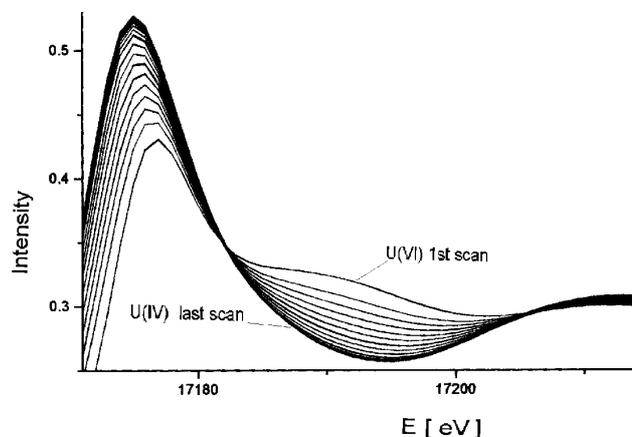
Fig. 2: U  $L_3$ -edge XANES spectra taken in situ during the reduction process
