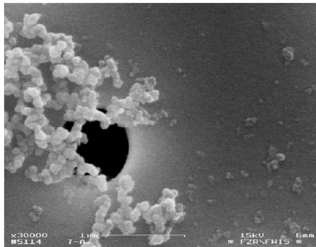
Fig. 2: SEM image (30000 x) of colloid particles and aggregates in the first batch, and pore of 1 µm filter membrane (Shot: E. Christalle).
