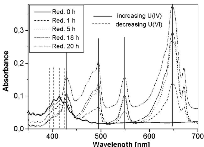
Fig. 3: UV/VIS spectra for reduction of uranium
