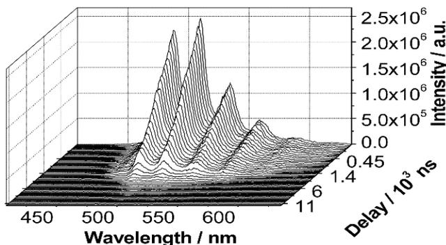
Fig. 1: Time-resolved fluorescence spectrum of uranium(VI)
