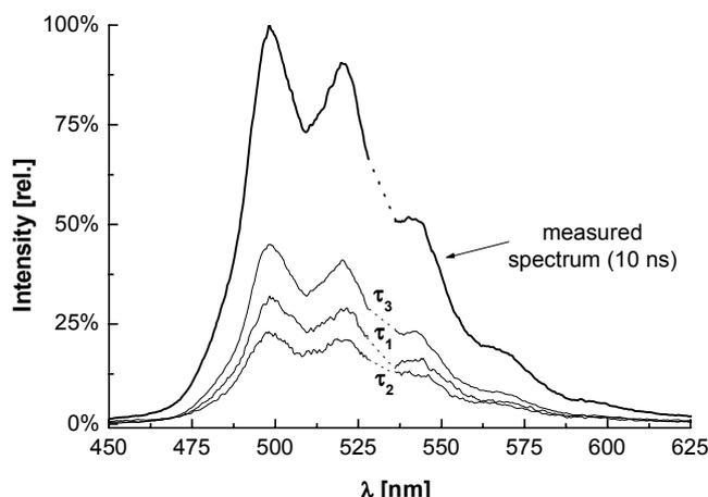
Fig. 2: Measured and deconvoluted fluorescence spectra of U(VI) sorbed on pyrophyllite
