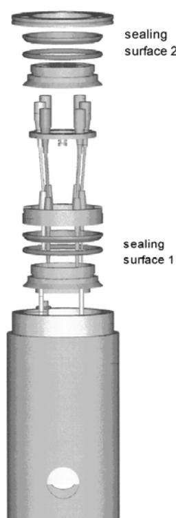
Fig. 1: Electrochemical cell (exploded design)
