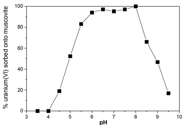
Fig.1: Sorption edge of uranium(VI) sorption onto muscovite at  $10^{-7} \text{ M } UO_2^{2+}$  and  $I = 0.1 \text{ M } NaClO_4$
