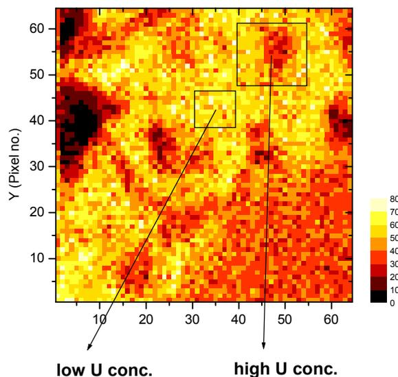
Fig. 2: Fe distribution within the chamosite chlorite in a region of  $250 \mu\text{m} \times 250 \mu\text{m}$ . Two areas with low and high U concentrations are shown.
