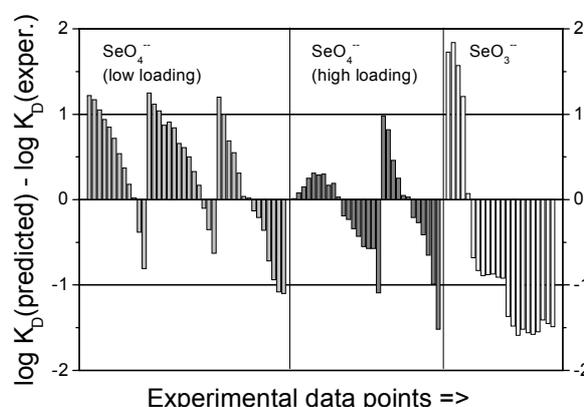
Fig. 1: Comparison of predicted and published experimental distribution coefficients for SeO<sub>4</sub><sup>2-</sup> and SeO<sub>3</sub><sup>2-</sup> with goethite
