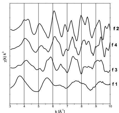
Fig. 1: Real spectral factors derived by ITFA, corresponding to the experimental XAFS spectra of franklinite (f 2), sphalerite (f 3) and Zn oxalate (f 1). Factor 4 corresponds to the XAFS spectrum of the previously undetected species, a Zn-Fe spinel (franklinite 2).
