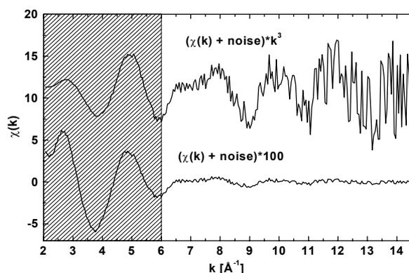
Fig. 2: k<sup>3</sup>- and k<sup>0</sup>-weighted EXAFS spectra of ac with artificial noise. Dashed – the optimum k-range for analysis.
