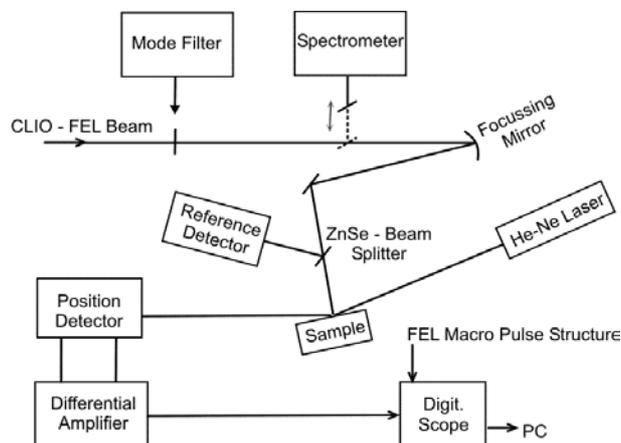
Fig. 1: Schematic diagram of the thermal deflection experiment setup.
