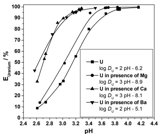
Fig. 1: Uranium extraction by  $LH_6$  in absence and presence of competing ions as a function of pH value. Organic phase:  $[LH_6] = 5 \times 10^{-4}$  M,  $CH_2Cl_2$ .
