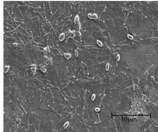
Fig.2: SEM picture showing the stage of adhesion of further bacteria to the attached microcolonies
