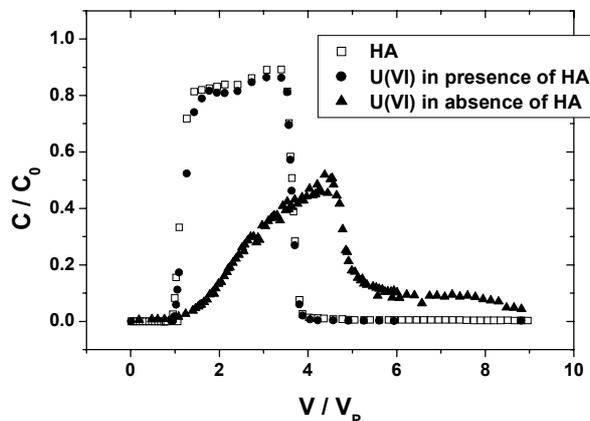
Fig. 1: Breakthrough curves of HA and U(VI). C: measured and C<sub>0</sub>: initial concentration. V: effluent volume, V<sub>p</sub>: effective pore volume.
