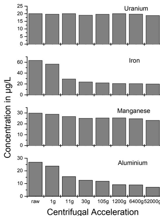
Fig. 1: Concentration of the key elements (stream, April 2003) in various centrifugates (centrifugation time: 1h)
