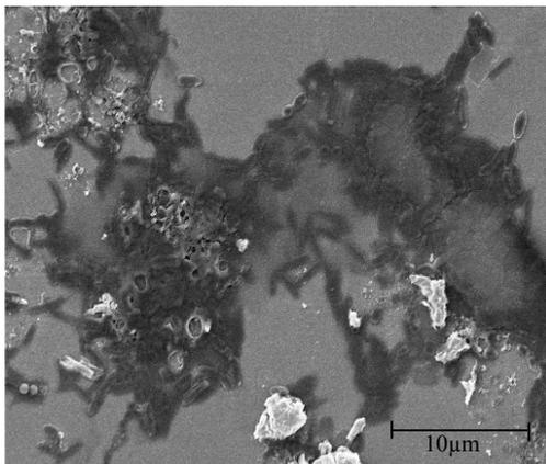
Fig.1: SEM picture showing the stage at which microcolonies are attached to the surface and the production of EPS has set in
