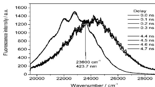
Fig. 3: Construction of the isoemissive point of a time-resolved spectrum
