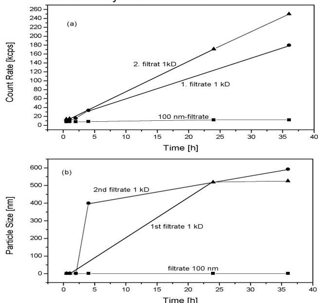
Fig. 1: Results of the PCS-measurements on the filtrates of the ARD-water, (a) the scattered light intensity (count rate) and (b) the particles size according to the deconvolution of the autocorrelation functions which was done with the CONTIN procedure.
