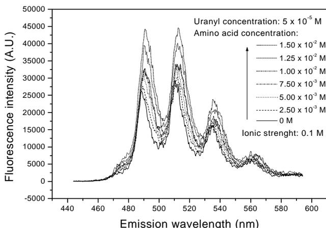
Fig. 1: Fluorescence spectra of uranium (VI) as a function of the L-threonine concentration at pH 4
