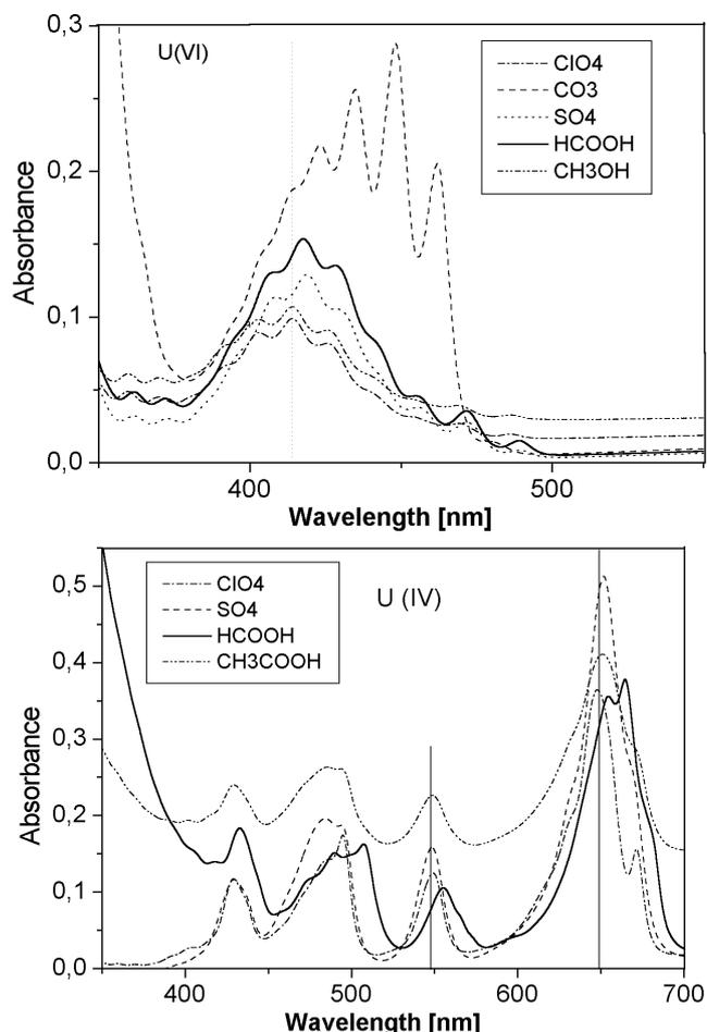
Fig. 2: UV/VIS spectra for U(VI) (stock solution) and U(IV) (completely reduced solutions) with various anions
