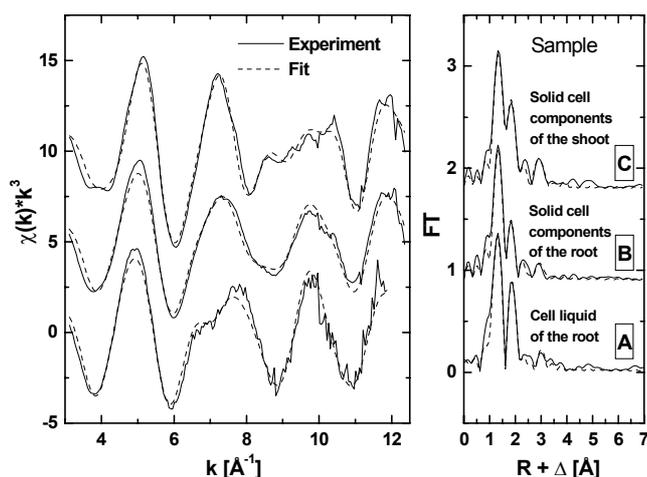
Fig. 1: Raw U  $L_{III}$ -edge  $k^3$ -weighted EXAFS spectra (left) and their corresponding Fourier transform (right) of investigated cell components.
