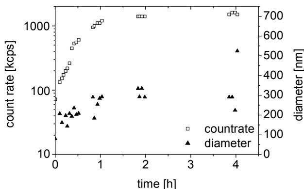
Fig. 2: Course of particle diameter (CONTIN deconvolution) and count rate in a 1h 52000 g centrifugate of sample FW-2.
