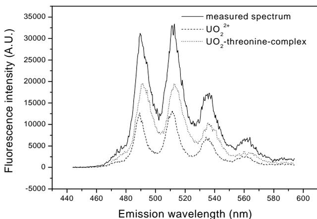
Fig. 2: Peak deconvolution of the fluorescence spectrum of a solution containing  $5 \cdot 10^{-5}$  M uranyl and  $5 \cdot 10^{-3}$  M L-threonine at pH 4.
