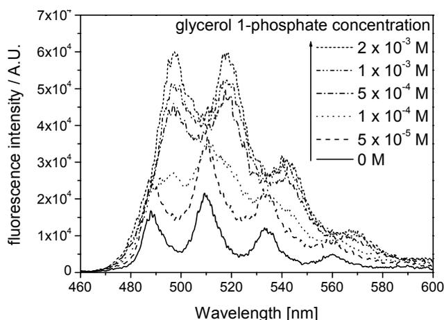
Fig. 1: TRLFS spectra of uranium(VI) ( $10^{-5}$  M) as a function of the ligand concentration at pH=4.0.
