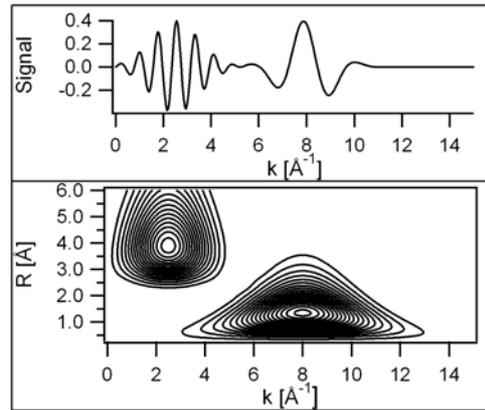
Fig. 3: Model function with distances  $r_1=4.0$  and  $r_2=1.3$  centered at  $k=2.5, k=8.0$  and the WT.
