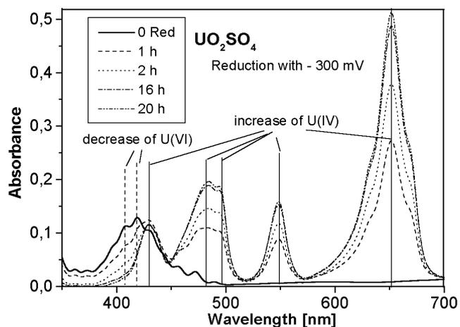
Fig. 1: UV/VIS spectra during reduction of 0.01M  $UO_2SO_4$ , 0,02 M NaCl, pH = 0,78 with  $H_2SO_4$
