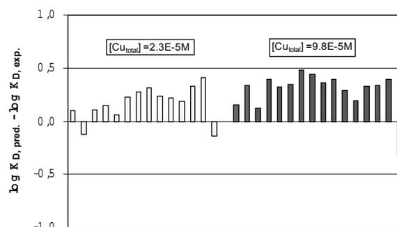
Fig. 2: Difference between predicted K<sub>D</sub> and experimental values
