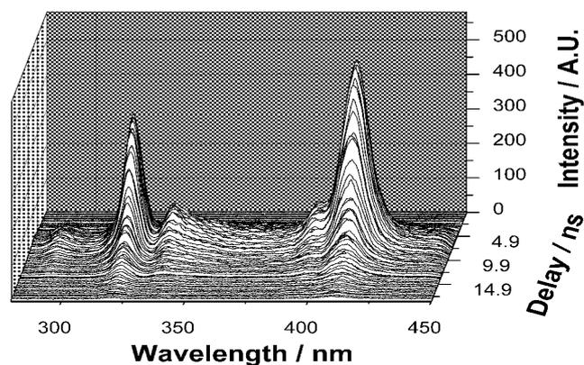
Fig. 2: Time-resolved fluorescence spectrum of uranium(IV) in perchloric acid
