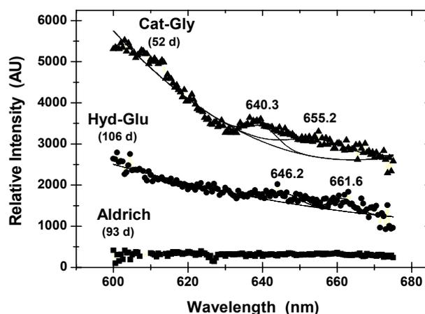
Fig. 1: Photoacoustic spectra of the studied HA solutions. Numbers in brackets indicate the equilibration time of the samples.
