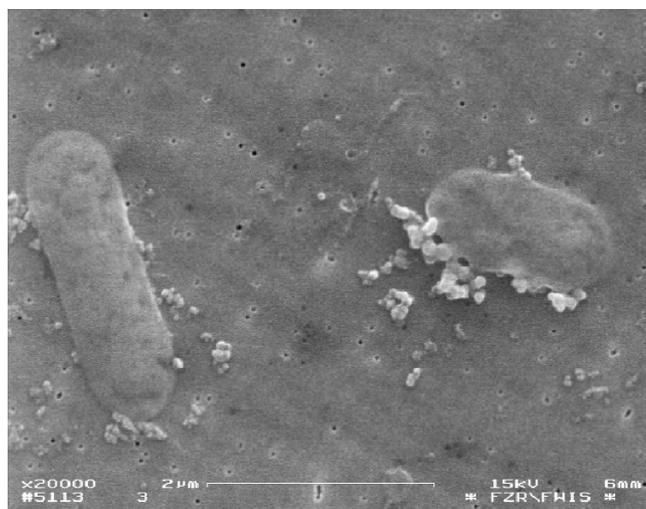
Fig. 3: SEM image (20000 x) of bacteria and colloids in FW-2 with 50 mL water filtered over a 50 nm membrane (Shot: E. Christalle).
