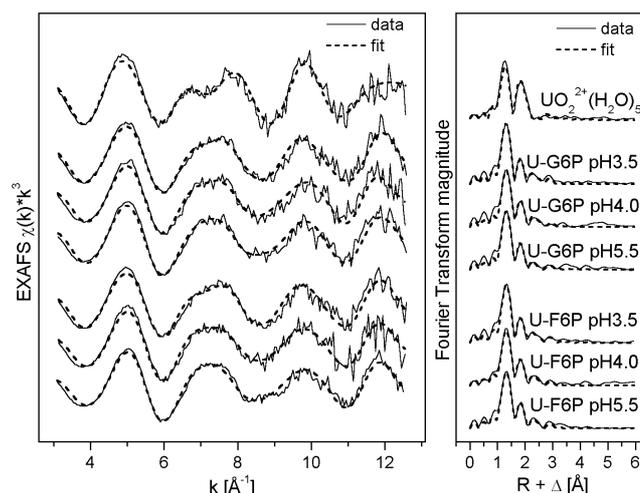
Fig. 1: Raw U  $L_{III}$ -edge  $k^3$ -weighted EXAFS spectra (left) and the corresponding Fourier transform (FT) (right).
