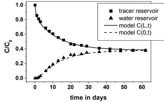
Fig. 2: HTO concentration in both reservoirs versus time
