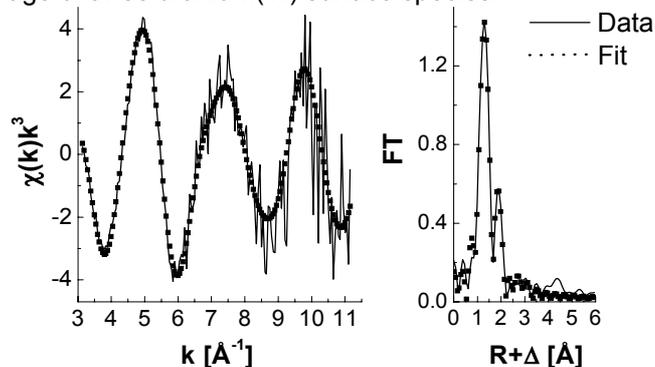
Fig. 3: U-L<sub>III</sub> edge EXAFS spectrum and Fourier transform of the uranium(VI) sorption sample
