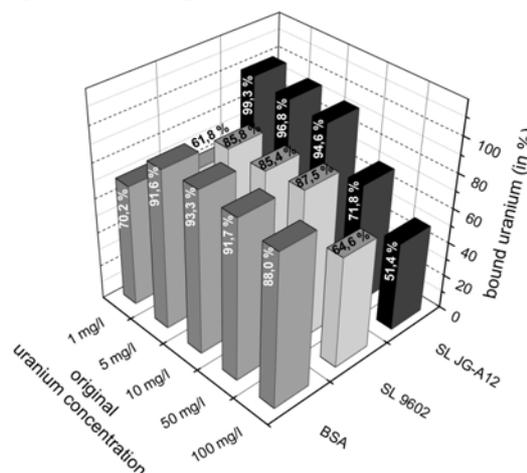
Fig. 2: Uranium binding of 1.5 g/l S-layer protein of the *B. sphaericus* strains JG-A12 and NCTC 9602 compared to that of 1.5 g/l serum bovine albumine.
