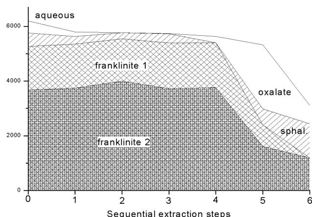
Fig. 2: Absolute species distribution (Zn in mg/kg, cumulative) of the untreated soil sample (step 0) and after each of the selective sequential extraction steps (1 to 6).
