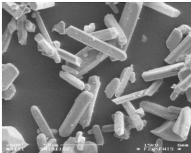
Fig. 1: SEM picture of a sample of synthetic swartzite
