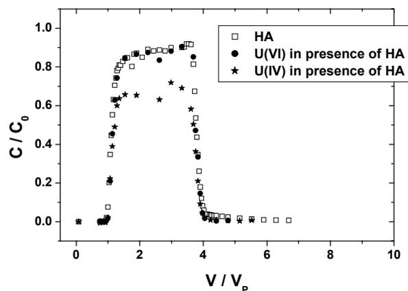
Fig. 2: Breakthrough curves of HA, U(IV) and U(VI).
