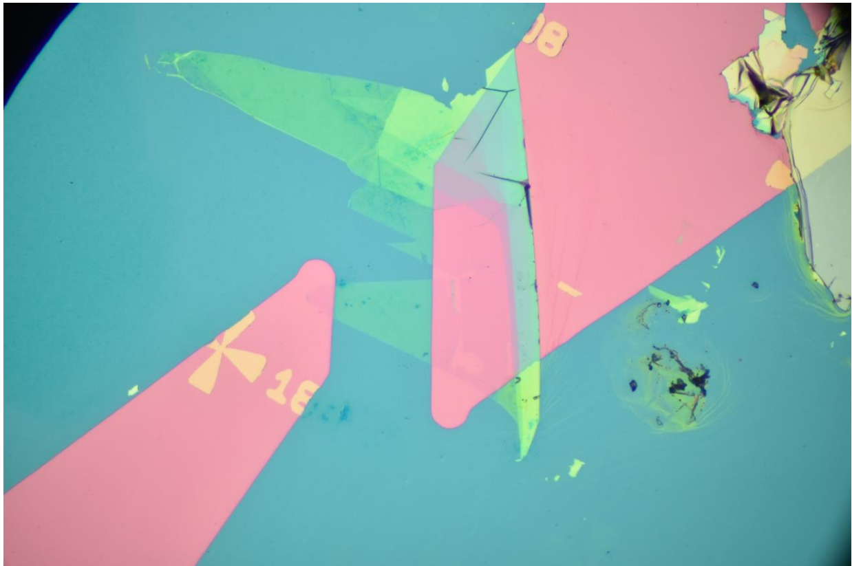
Figure 1 Optical microscope image (50x magnification) of a WS 2 monolayer flake contacted with a thin gold film.
