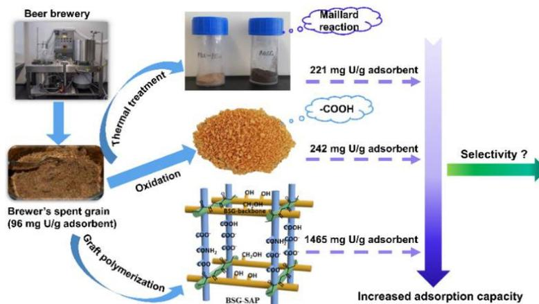
Figure 42 Preparation of adsorbents for uranium adsorption from BSG through thermal treatment, oxidation, and graft polymerization.
