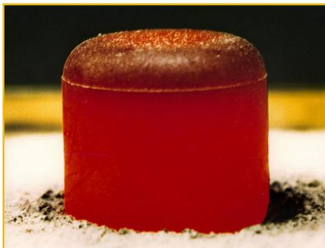
Figure 1. 150g sintered  $^{238}\text{PuO}_2$  General Purpose Heat Source pellet.
