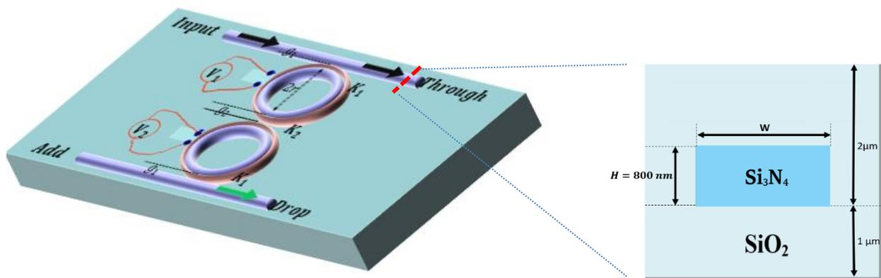
Figure .1 a) Schematic of a coupled-resonator optical waveguide (CROW) filter in SiN platform, which consists of two identical rings, each with a coupling coefficient  $\kappa_1$  between the rings and the bus waveguides and coupling coefficient  $\kappa_2$  between the rings themselves. b) Waveguide cross section.
