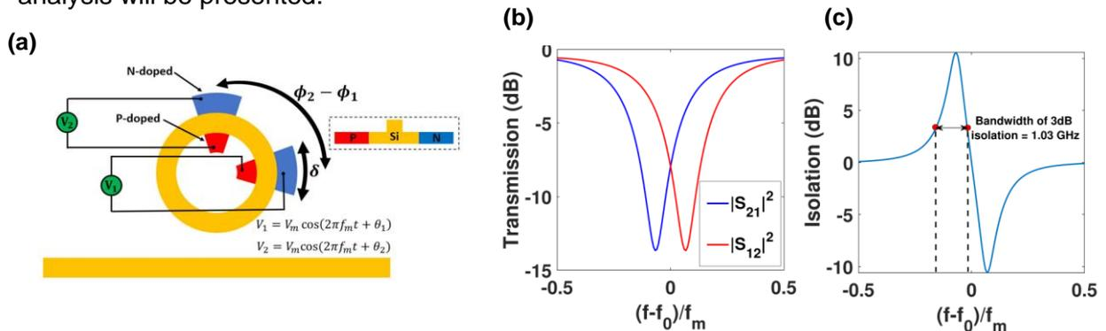
Fig. 1. (a) Ring resonator with two time-modulated point perturbations, side coupled to the bus waveguide. (b) Forward ( $S_{12}$ ) and backward ( $S_{21}$ ) power transmission spectrum of the time-modulated ring resonator and, (c) optical isolation ( $|S_{12}|^2/|S_{21}|^2$ ) versus frequency.
