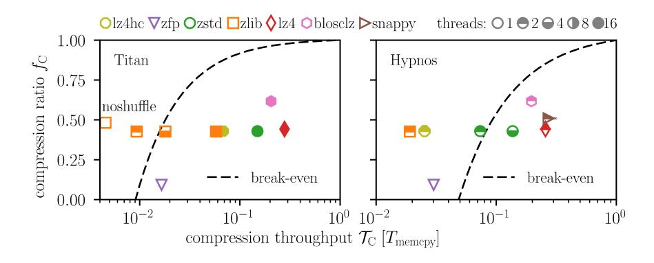
Zfp 0.5.1: three uncompressed bits / scalar; on particle data
