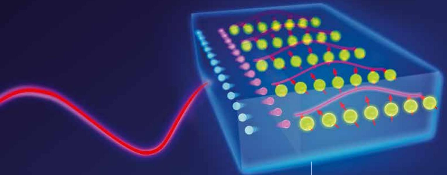
In a magnet sandwich made of thin metal layers, a terahertz light wave (from left) is converted into a spin wave.
