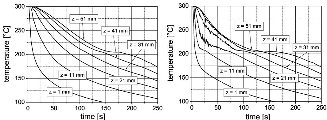
Figure 10 Cooling curves obtained inside a Pb85 wt%Sn alloy solidified directionally. Left: without electromagnetic stirring; right: under the influence of an RMF ( $B = 10$  mT,  $f = 50$  Hz,  $Ta = 1.7 \times 10^7$ ).
