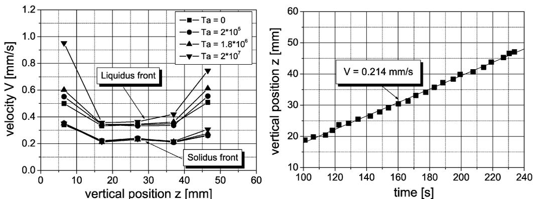
Figure 12 Growth velocities of liquidus and solidus front calculated from temperature data (left), and of the solidification front determined by UDV (right) under the influence of an RMF (right: *B* = 10 mT, *f* = 50 Hz, *Ta* = 1.7 × 10<sup>7</sup>).
