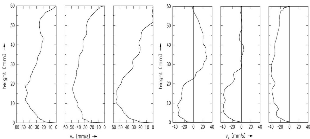
Figure 8 Snapshots of vertical velocity profiles. Left: upward directed TMF ( $B = 7$  mT,  $f = 70$  Hz,  $Ta = 9.7 \times 10^6$ ) measured at a radial coordinate of 18 mm; right: combination of a downward travelling field with same parameters as in left graph and an RMF ( $B = 3.5$  mT,  $f = 70$  Hz,  $Ta = 2.4 \times 10^6$ ), measured in the centre.
