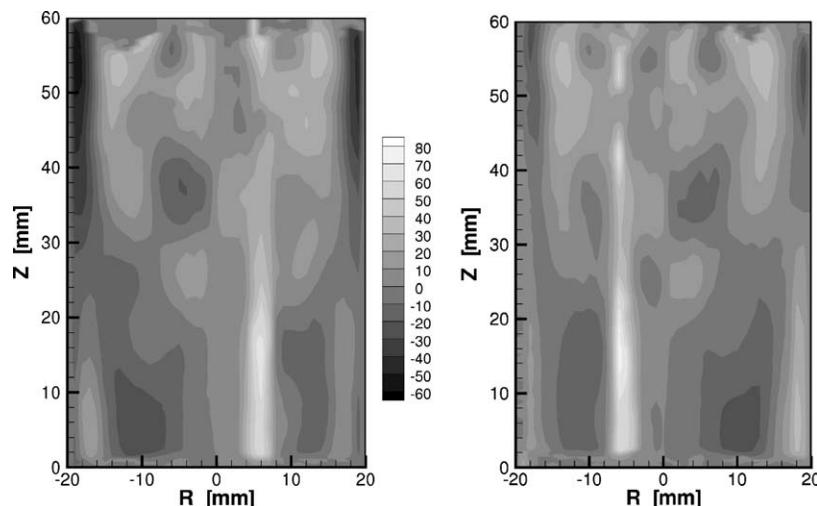
Figure 6 Iso-contour plots of the vertical velocity component of a flow driven by a RMF ( $f = 50$  Hz,  $B = 9.2$  mT,  $Ta = 9.5 \times 10^6$ ). The legend of the velocity scale is in mm/s, positive values represent a downward flow. Left: radial movement of the transducer along an arbitrary axis; right: radial direction changed by  $90^\circ$ .
