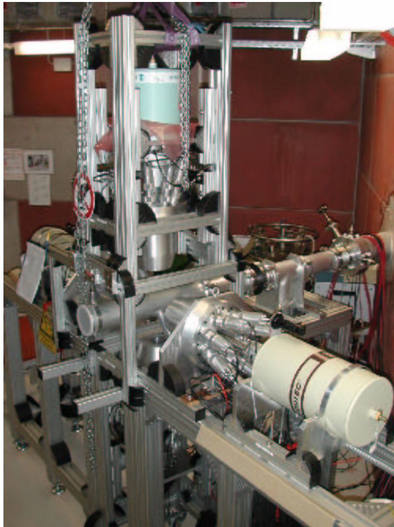
Fig. 1 Setup of high-purity Ge detectors surrounded by escape-suppression shields. The photon beam enters the experimental area from the right.
