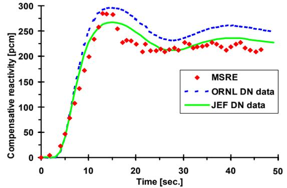
Fig. 5: Compensative reactivity inserted by the fuel pump start-up transient (constant power is maintained). Original ORNL DN data and calculated JEF DN data were used.
