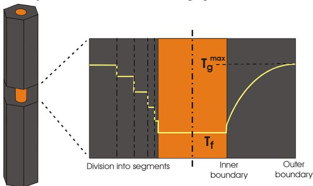
Fig. 3: Modeling of the temperature distribution in a graphite channel by 5 segments with effective heat transfers coefficients. Comparison of the calculated steady state distribution (on the left) with analytical solution (on the right).
