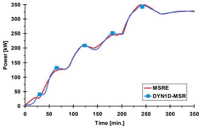
Fig. 7: The power history during the 350 minutes of the natural circulation experiment (U233/U235/Pu239 fuel).
