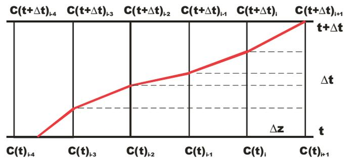
Fig. 1: Path of fictitious fluid particle during one time step  $\Delta t$  through several nodes with different fuel velocity to the edge of the  $i$ -th node.
