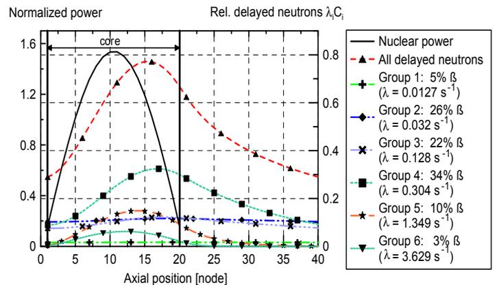
Fig. 2: Distribution (normalized to 1) of power (left scale) and of 6 groups of delayed neutrons (right scale) for flowing fuel reactor  $v \approx 1\text{m/s}$ .
