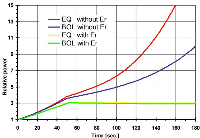
Fig. 10: MSBR response to the fuel overcooling by 50°C at the core inlet for four different cross-sections libraries.
