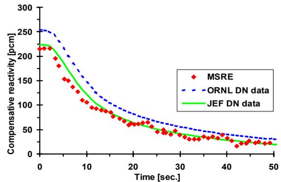
Fig. 6: Compensative reactivity inserted by the fuel pump trip transient (constant power is maintained). Original ORNL DN data and calculated JEF DN data were used.
