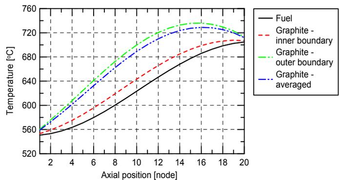
Fig. 4: Typical axial distributions of temperature in the steady state for the fuel channel of MSR. The fuel temperature at the core inlet is 550°C. Flowing through the core; it is heated up by 150°C approximately.
