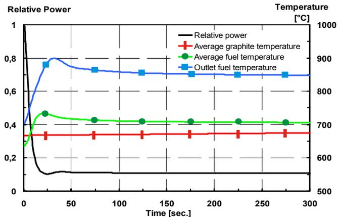
Fig. 8: MSBR response to the unprotected fuel pump trip. The power is sharply decreased because of the strong negative feedback coefficient of the fuel salt. (used library: EQ with Er)
