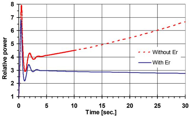
Fig. 9: MSBR response to the 300 pcm reactivity insertion.
