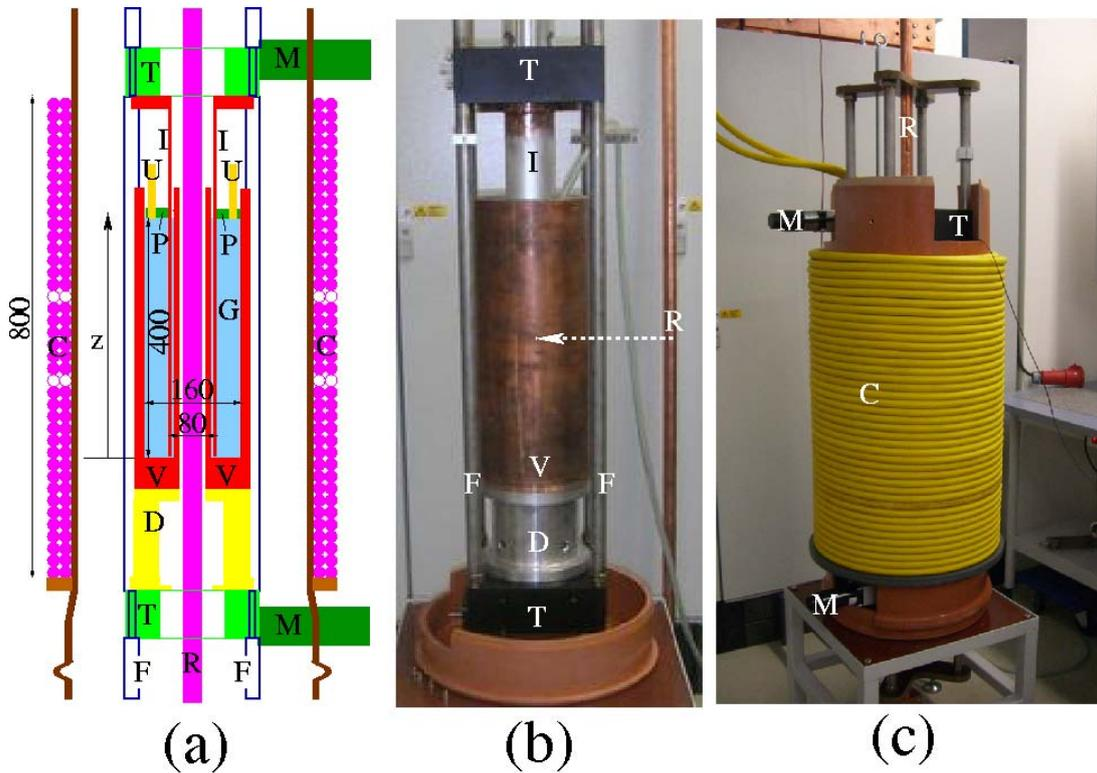
Fig. 1: The PROMISE experiment. (a) - Sketch. (b) - Photograph of the central part. (c) - Total view.  $V$  - Copper vessel,  $I$  - Inner cylinder,  $G$  - GaInSn,  $U$  - Two ultrasonic transducers,  $P$  - Plexiglas lid,  $T$  - High precision turntables,  $M$  - Motors,  $F$  - Frame,  $C$  - Coil,  $R$  - Copper rod. The dimensions are in mm.
