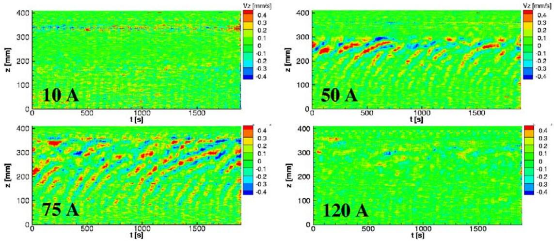
*Fig. 2: Measured axial velocities in dependence on the vertical position and the time, for different coil currents. The appearance and disappearance of a travelling wave mode for increasing coil current (i.e., Hartmann number) is clearly visible.*
