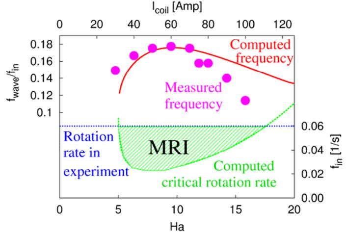
Fig. 4: Computed critical rotation rate for varying  $I_{coil}$  (and hence  $Ha$ ), for fixed  $I_{rod} = 6000$  A, and measured and computed frequency  $f_{wave}$  of the travelling MRI wave normalized to  $f_{in}$ .
