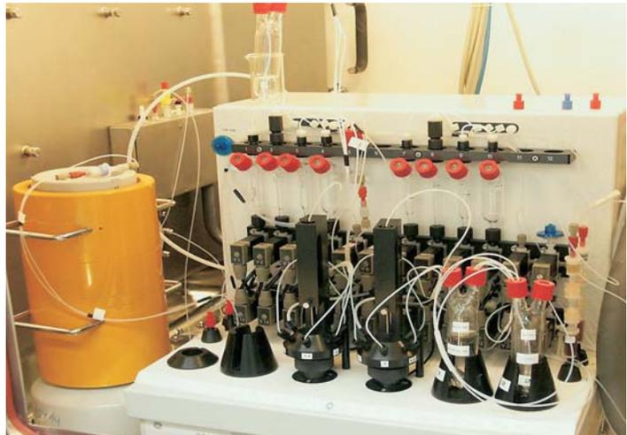
The radiosynthesis of [ $^{18}\text{F}$ ]fluoroacetate was developed in course of a diploma thesis. The synthesis is performed in a remotely-controlled, well-shielded synthesis module. [ $^{18}\text{F}$ ]Fluoroacetate can be prepared very reliably as a robust two-step/one-pot synthesis sequence in good radiochemical yields and very high radiochemical purity.
