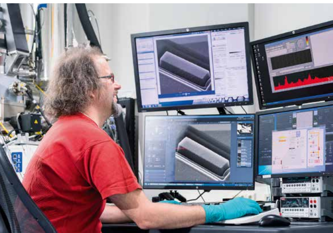
With the help of a helium ion microscope, physicist Gregor Hlawacek can trim nanometer-sized samples into the desired form. Source: A. Wirsig
