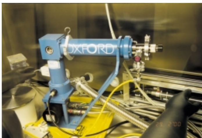
Fig. 1: View into the ROBL glove box: special designed helium cryostat (OXFORD Instruments) with horizontally arranged sample holder.
