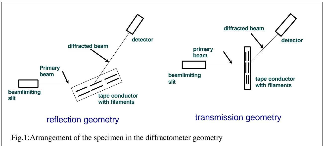
Fig.1: Arrangement of the specimen in the diffractometer geometry
