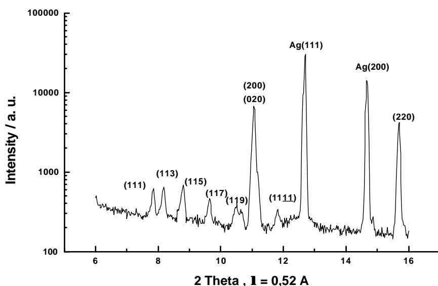
Fig.3: diffraction pattern recorded in transmission geometry
