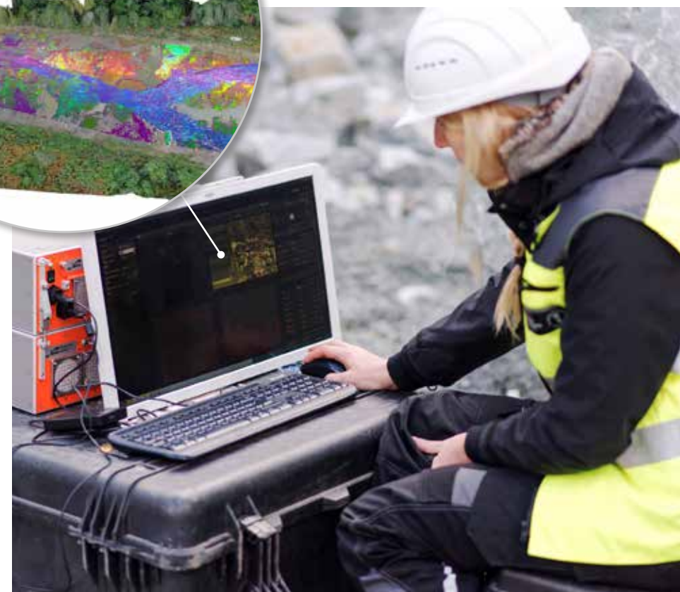
While still in the field, models of the terrain can be created using the data collected from hyperspectral cameras. The different colors provide information about different mineral contents. ©HZDR/HIF
