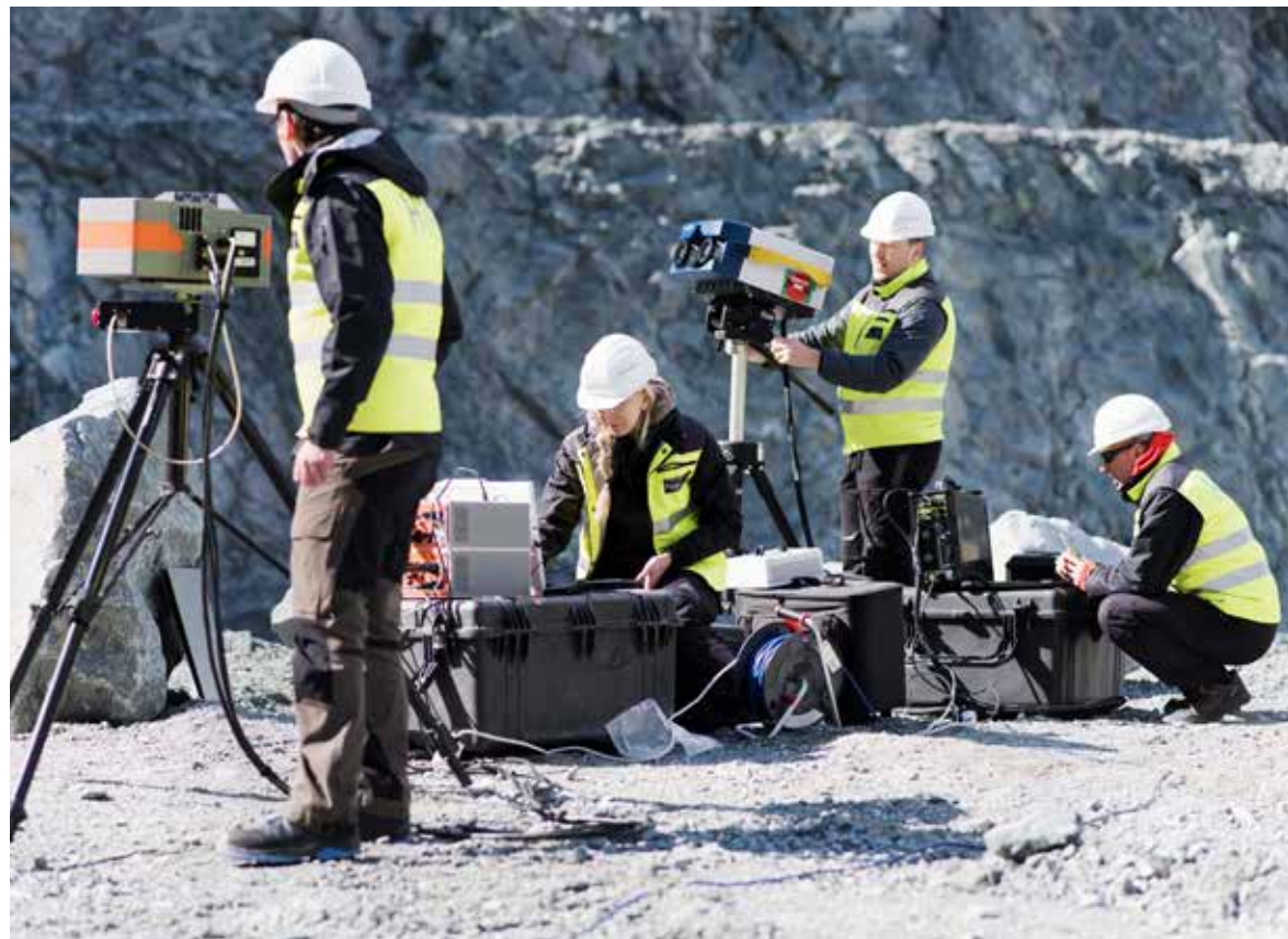
Geologists can view and evaluate the images taken by the hyperspectral cameras directly in the field. ©HZDR/HIF
