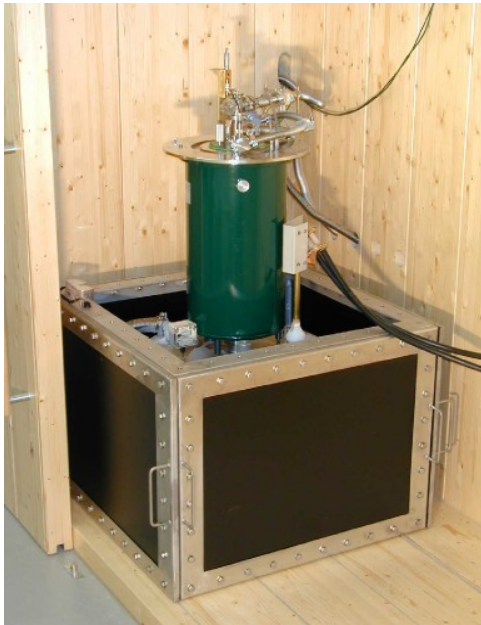
Cryostat and coil inside armored box Capacitor bank: 4 modules, total energy 1 MJ at 10 kV
