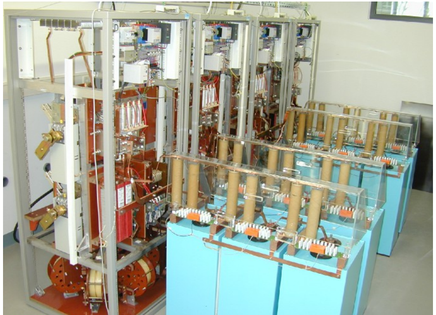
Cryostat and coil inside armored box Capacitor bank: 4 modules, total energy 1 MJ at 10 kV
