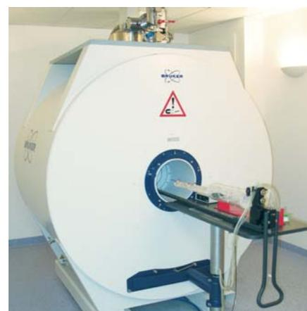
**Fig. 2:** Small animal magnetic resonance tomograph with a magnetic field strength of 7 Tesla (BioSpec 70/30, Bruker BioSpin MRI GmbH, Ettlingen, Germany).
