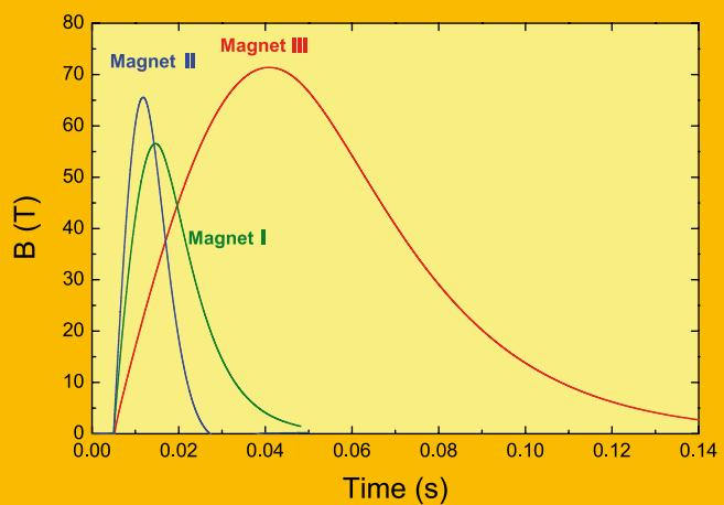
At the moment, the HLD operates three types of user magnets with the above shown temporal field profiles.
