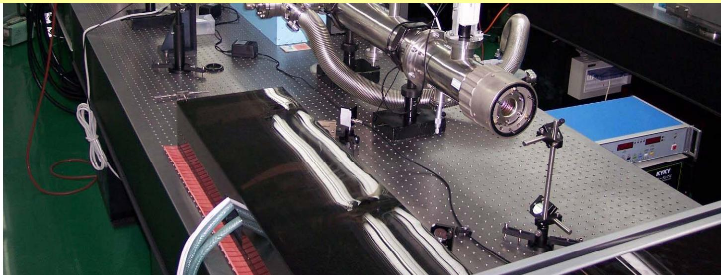
This system is based on CPA scheme, with a peak power of 890TW and a pulse duration of 29fs. It consists of a Ti:sapphire oscillator, a pulse stretcher, four stages of amplifiers and a four-grating pulse compressor.
